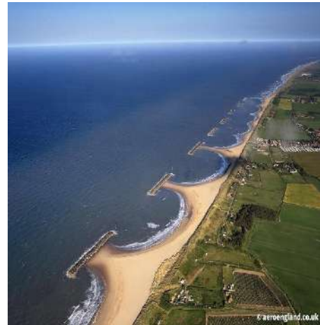
Slika 20. Valobran povezan sa obalom ( https://aeroengland.photodeck.com/media/191cc356-53bd-4be1-9c5d-139b95415063-aerial-photograph-of-artificial-reef-offshore-breakwater-at-s )
