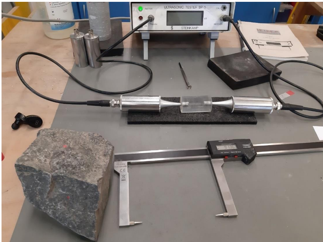
Figure 26 Ultrasonic testing device for P-wave velocity during calibration, distance measuring device and basalt sample.
