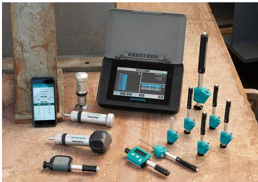
Figure 27 Equotip device (Proceq).
