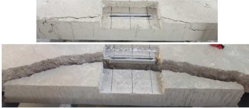
Figure 6.5 Breakout pattern for anchor channels installed in pockets - c_1 = 100 mm (upper) and c_1 = 200 mm (lower)
