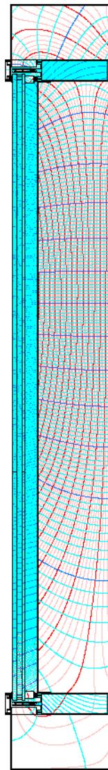
Figure 3. Heat flow lines (increment 0.1 W/m).
