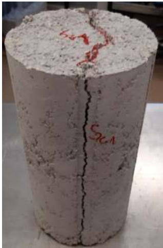
a) Typical failure mode
