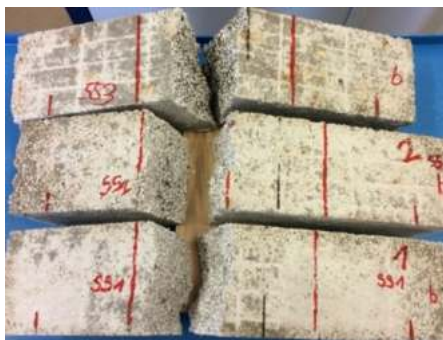
a) Typical failure mode
