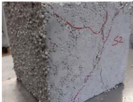
Figure 8. Compression test - failure patterns
