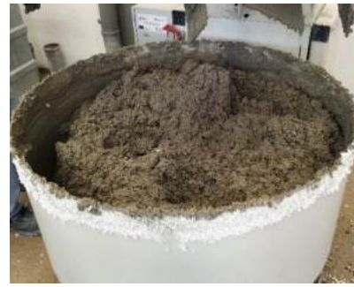
Figure 2. Fresh concrete mixture
