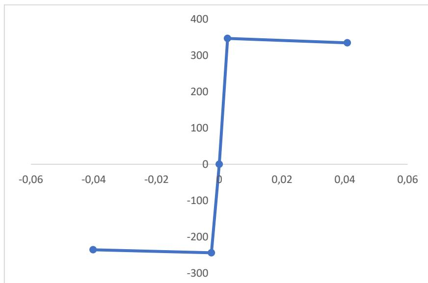
Slika 35. Dijagram M –  $\Theta$  greda 115-115 (ovijeni beton)
