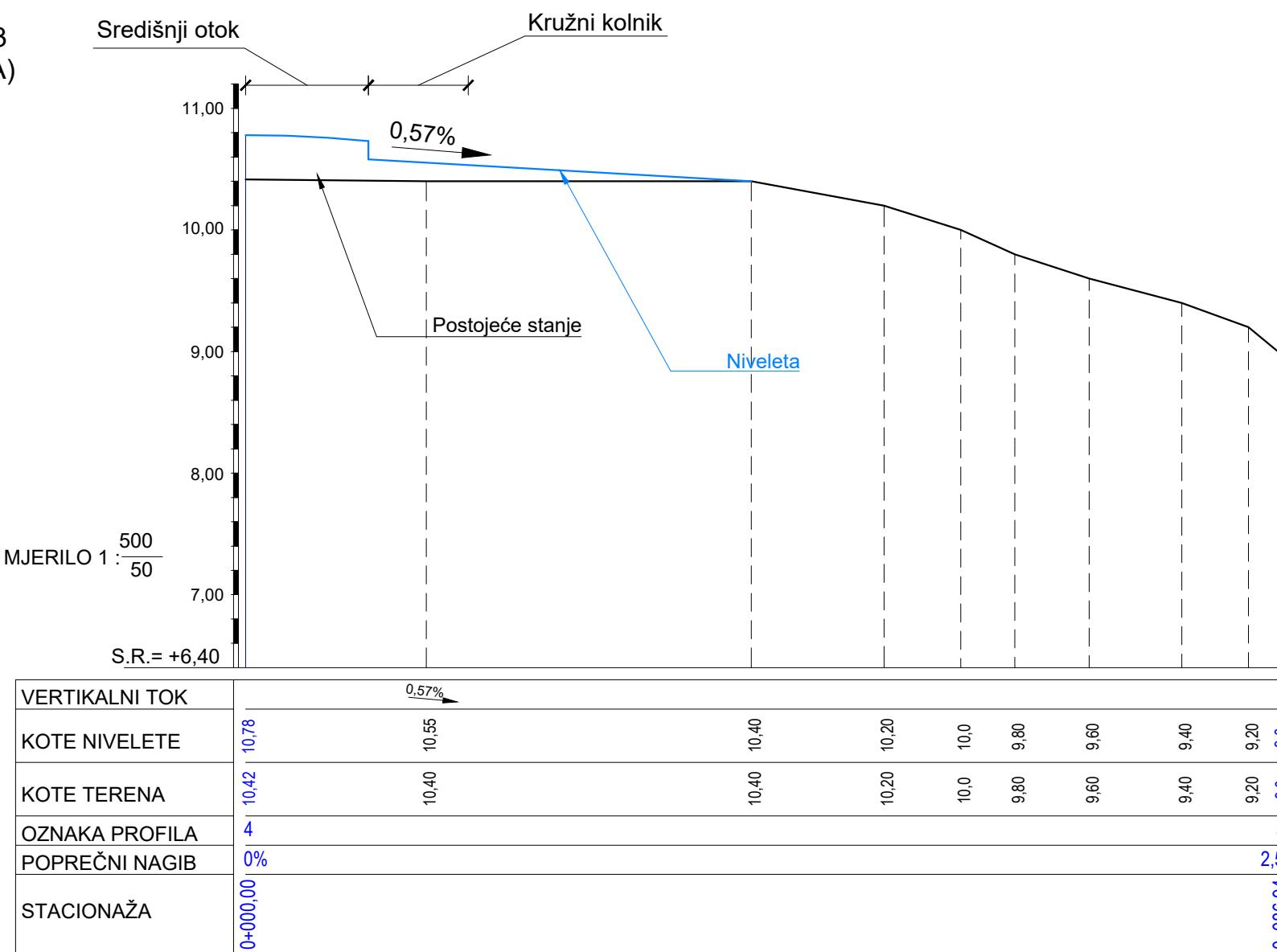
UZDUŽNI PRESJEK KRUŽNOG
