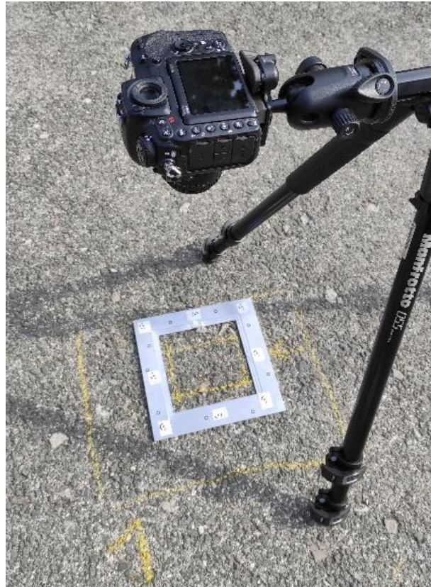
Figure 6.4 Texture data acquisition procedure by CROP methodology
