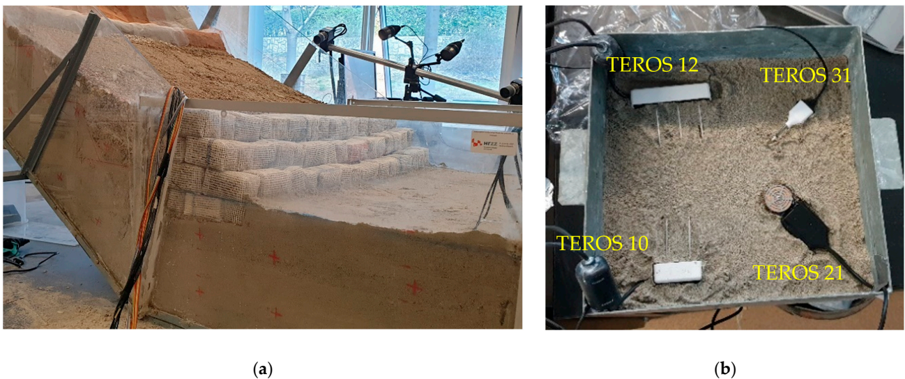
Figure 5. Details on (a) model setup with installation of sensors and cameras and (b) TEROS 12, 10, 31 and 21 sensors (top and bottom left and right, respectively) for hydraulic monitoring of slope models during the calibration procedure.
