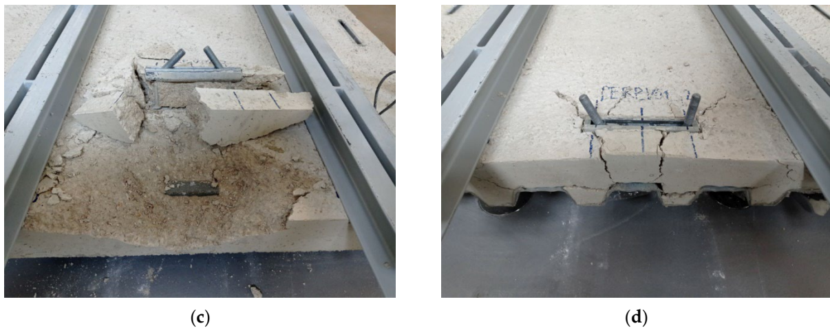
Figure 14. Breakout patterns for: (a) configuration 1; (b) configuration 2; (c) configuration 3; and (d) configuration 4.
