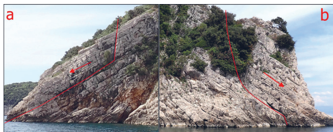
Figure 5. Structural interpretation of a possible slide in layered Upper Cretaceous limestones: a) south side, b) north side. Both red arrows are oriented to the east.
