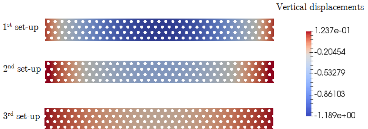
Figure 5.8: Plotted numerical results for vertical displacement field of B4 model [mm].
