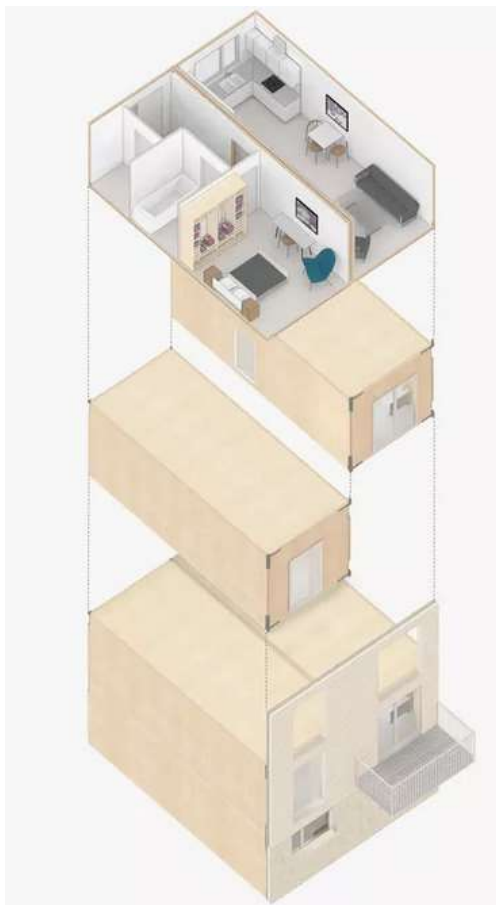
Slika 8: CLT 3D modularna konstrukcija (izvor: https://www.treehugger.com/construction-revolution-continues-cross-laminated-timber-goes-modular-4858141 , 26.05.2024.)
