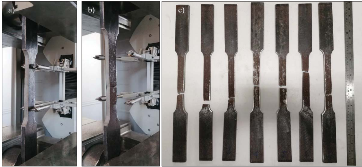
Figure 12. a) Testing setup; b) Specimen 7 just after fracture; c) Specimens after testing.
