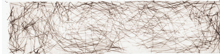
Figure 4.18: X-ray image of a fiber-reinforced concrete specimen [68].
