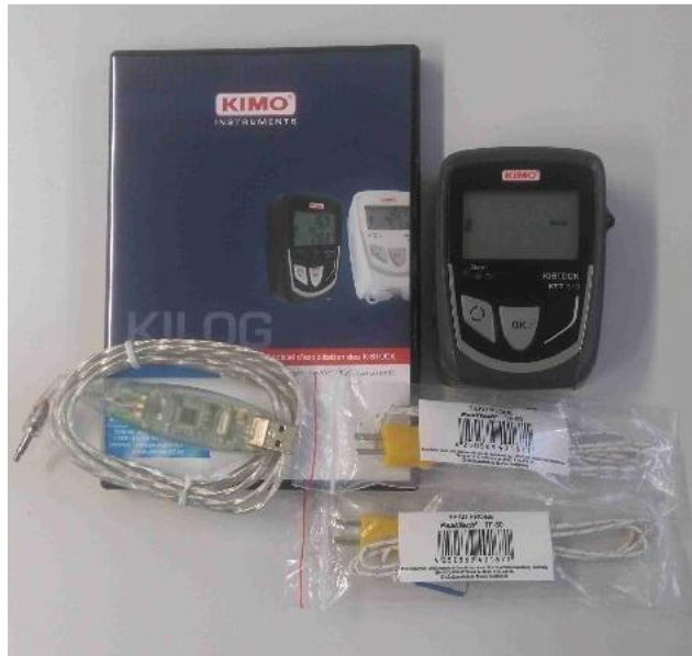
Slika 6. KIMO KISTOCK KTT310SET s sondama P TF-50
