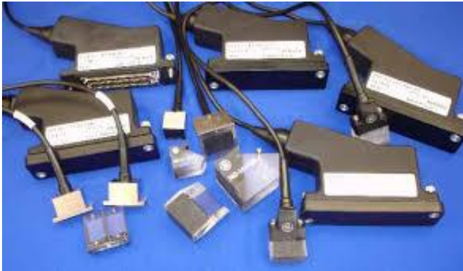
Slika 49: Phased array sonde [25]
