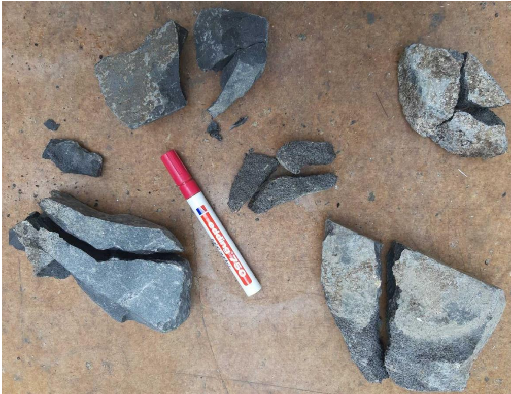
Figure 44 Samples after the Point Load Test.
