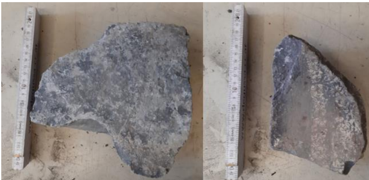
Figure 42 Basalt samples used for Schmidt hammer test
