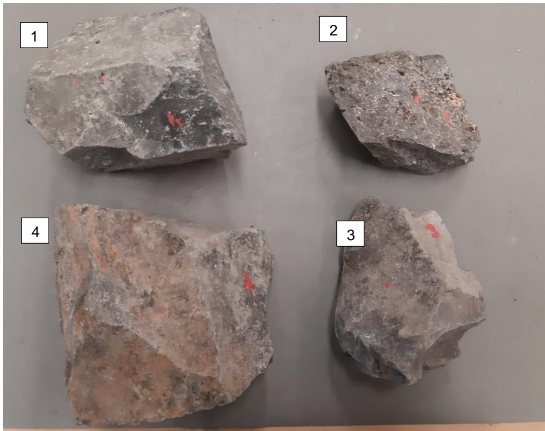
Figure 40 Basalt samples used for P-Wave velocity test.
