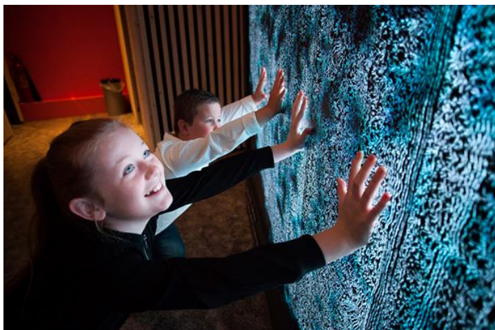
Slika 38: Betonski blok LiTraCon [ http://www.litracon.hu/en/products ]
