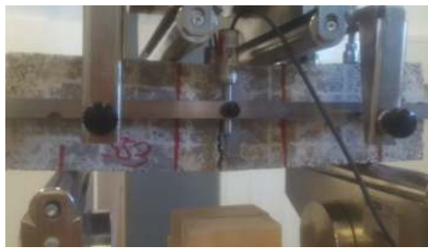
c) Crack initiation
