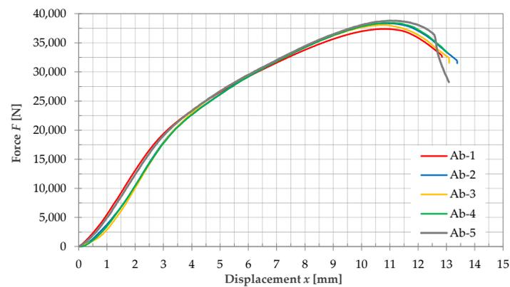
Figure 13. Force–displacement curves for the test specimens.
