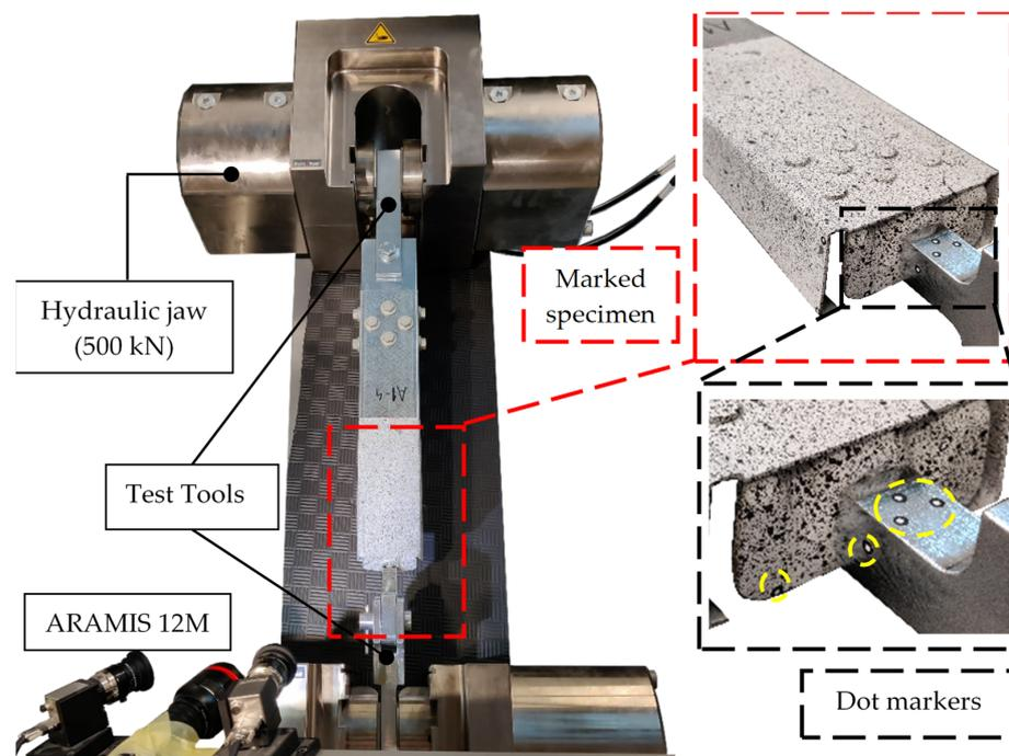
**Figure 10.** Test setup with DIC measuring system.
