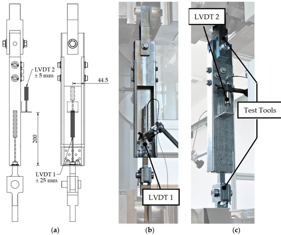
**Figure 9.** Test setup with (a) positions of LVDT devices on test specimen (mm) at (b) back view and (c) front view.
