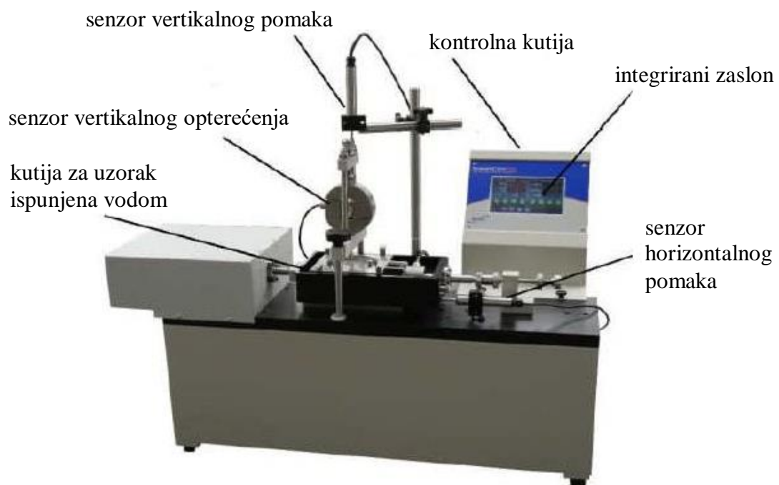
Slika 8: Uređaj za izravno smicanje (modificirano prema https://www.vjtech.co.uk/blog/an-introduction-to-direct-shear-testing )
