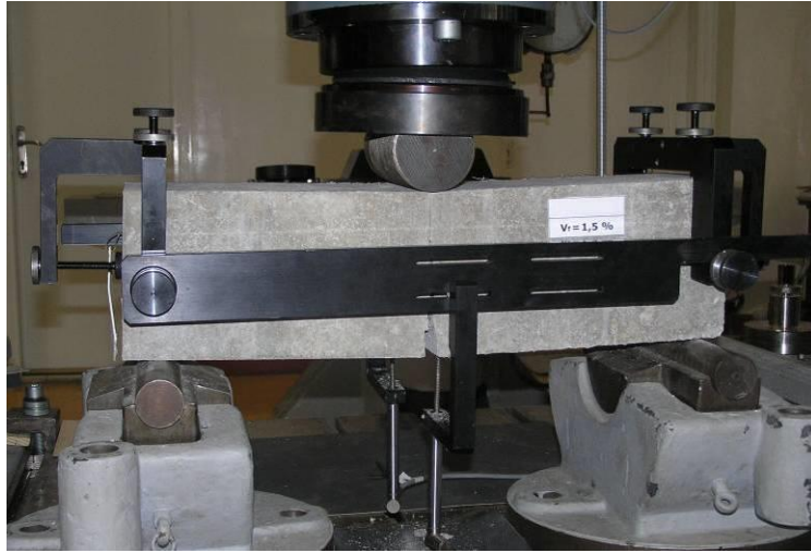
Fig. 5 Displacement controlled flexural 3-point bending test set-up ( V_f=1.5\% )
