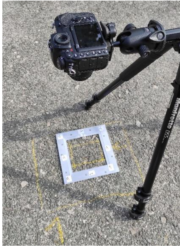
Figure 6.4 Texture data acquisition procedure by CROP methodology
