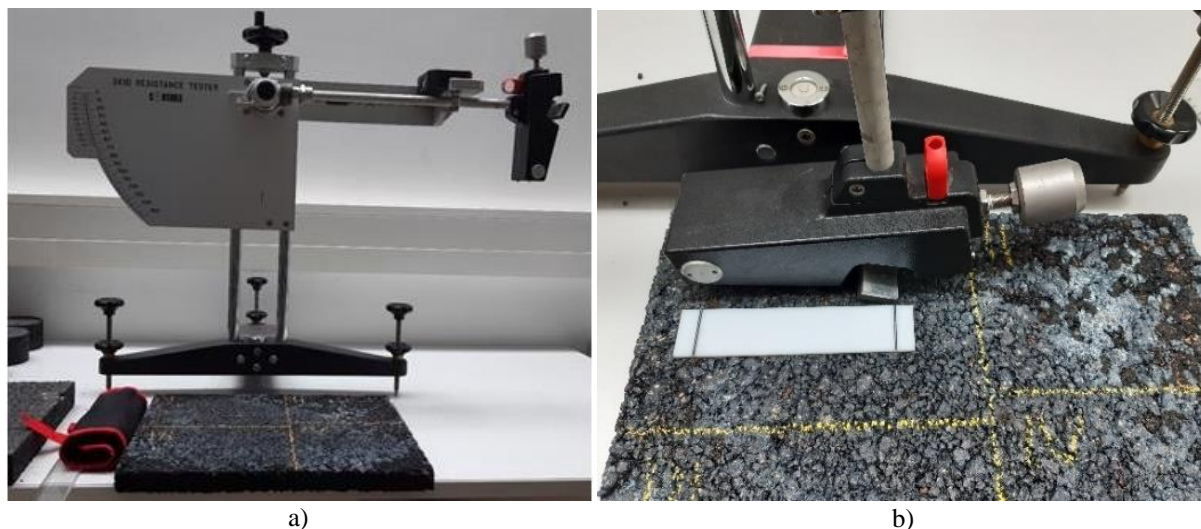
Figure 5.2. SRT low-speed friction measurement device (a) and friction measurement assembly on produced asphalt specimen (b)
