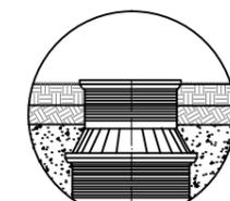
DETALJ UGRADNJE PE OKNA U TRAVNATE POVRŠINE
