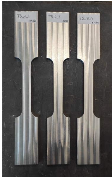
Figure 6.2: Test specimens (TS) for determination of material properties.
