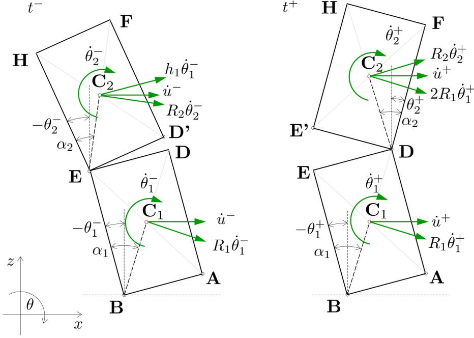
Figure 6.14: Velocity diagrams in configurations 1a and 2a
