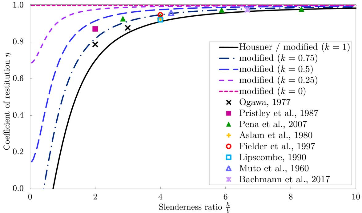
Figure 4.6: Coefficient of restitution from Housner’s formula [1], modified formula [2, 3] and previous experiments [34, 35, 36, 37, 38, 39, 40, 41]
