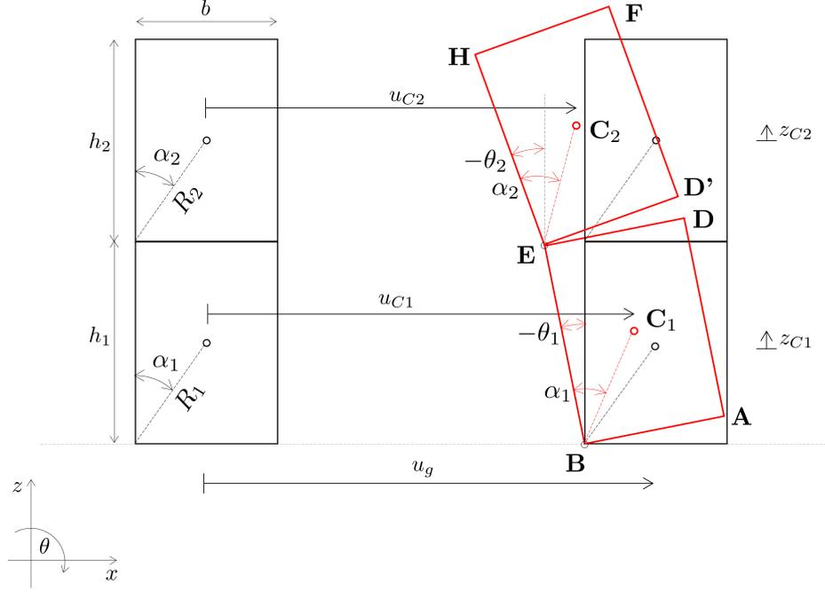
Figure 6.3: Displacements of the dual-block stack: translation and rotation in configuration 1a
