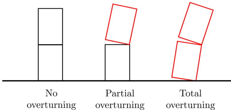
Figure 7.1: Modes of overturning of a dual-block stack
