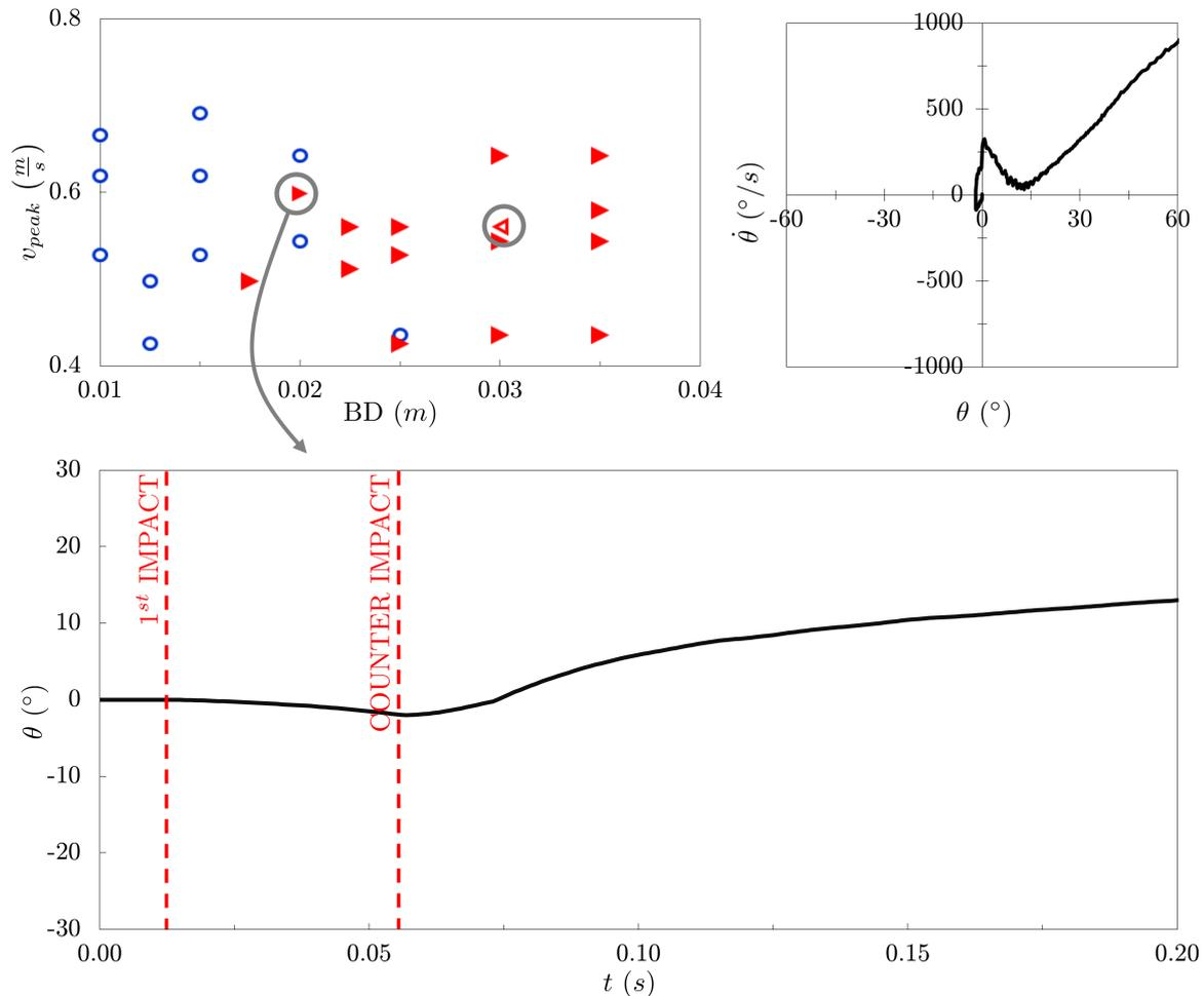
Figure 8.9: Phase plane view (above on the right) and rotation time history (below) of the experiment of a single block (Scale 1) motion with initial conditions  $v_{peak} = 0.59 \frac{m}{s}$ ,  $BD = 2.0 \text{ cm}$
