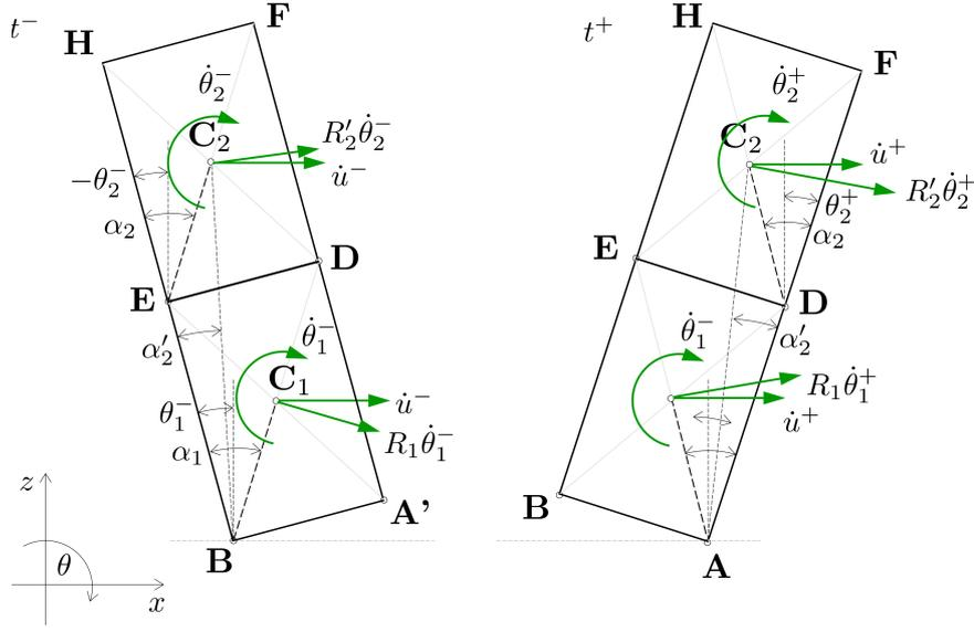
Figure 6.13: Velocity diagrams in configurations 3a and 3b
