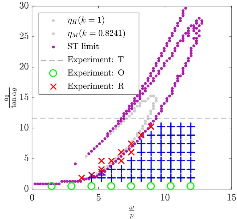
Figure 5.17: Stability graph due to a single sine wave for block B6M with  $h/b = 4.5$  (T - translation, O - overturning, R - rocking)
