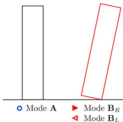
Figure 8.5: Modes of overturning of a single block
