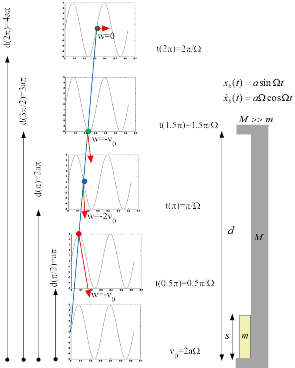
Figure 9.1: Rigid block, elastic collision. Maximum rebound velocity corresponds to a distinct geometry  $d = s + 2u_0\pi(1 + 2n)$ ,  $n = 0, 1, 2, \dots$  between the container basin size  $d$  and the excitation amplitude  $u_0$ . This relationship is independent of the excitation frequency
