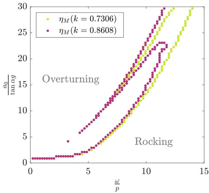
Figure 5.10: Stability graph for a single sine wave acceleration excitation for blocks with  $\frac{h}{b} = 4.5$ : B6M and B6L
