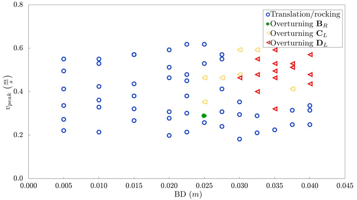
Figure 8.12: Modes of overturning of a three/block stack (scale 1) obtained from the experimental study
