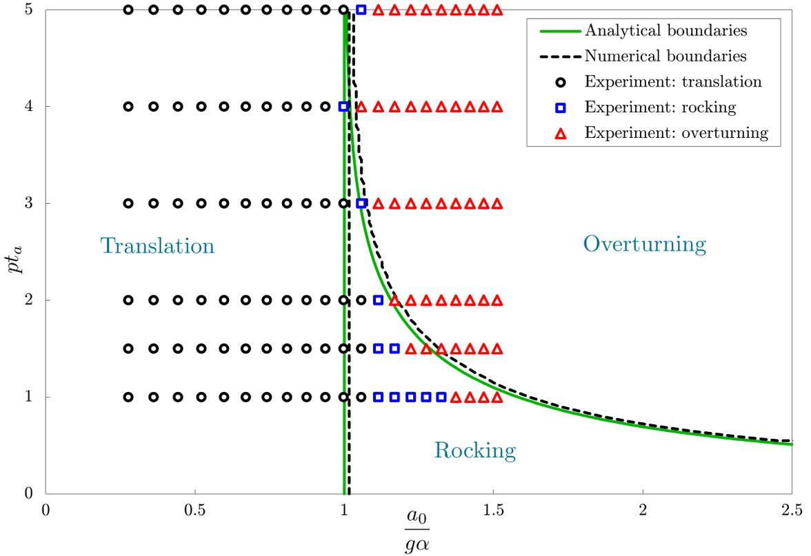
Figure 5.6: Experimental results for overturning/rocking/translation of the block due to a constant acceleration of finite duration
