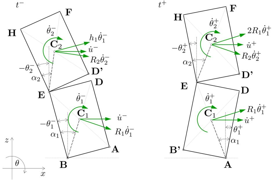
Figure 6.16: Velocity diagrams for configurations 1a and 2b
