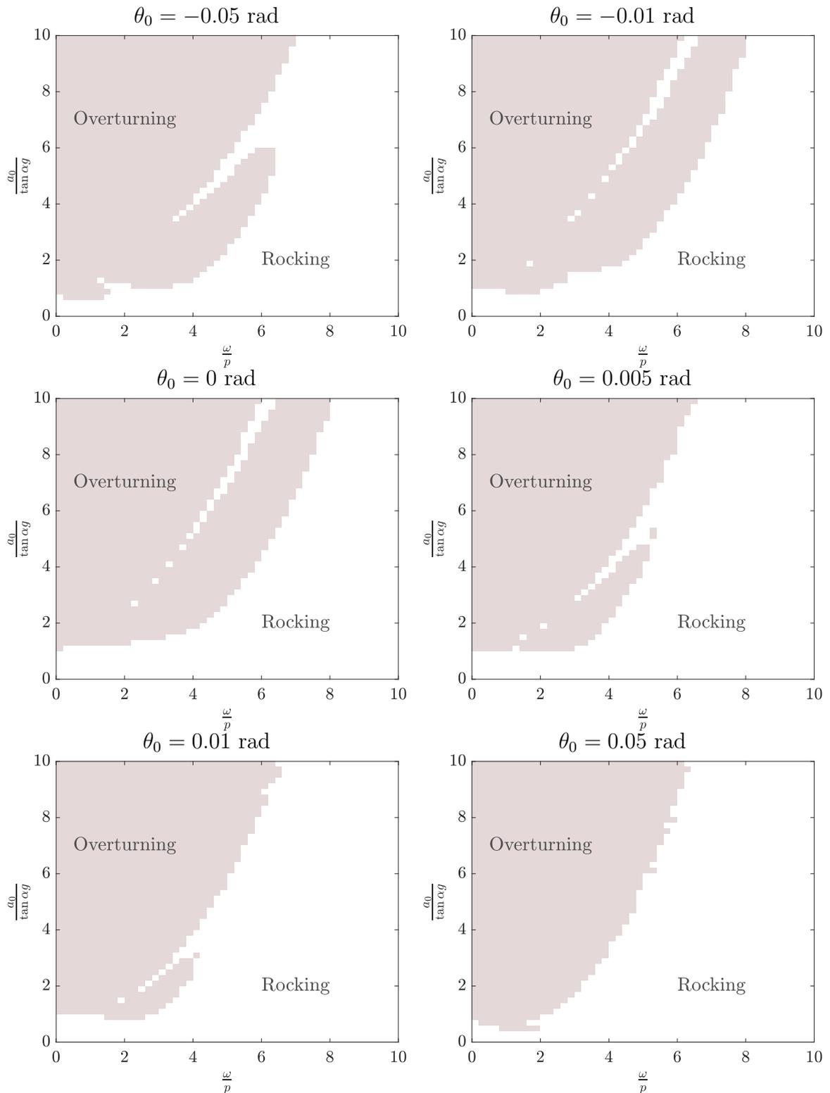
Figure 3.25: Overturning/non-overturning area depending on frequency and amplitude of ground acceleration function obtained during 10 seconds of nonlinear analysis of rocking motion of a slender rigid rectangular block with various initial rotation
