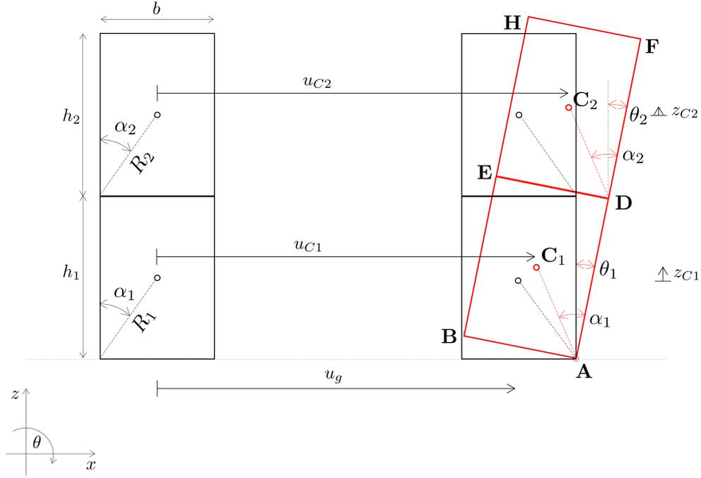
Figure 6.8: Displacements of the dual-block stack: translation and rotation in configuration 3b
