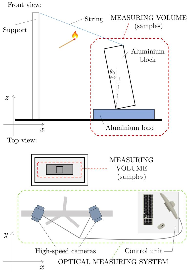
Figure 4.9: The free-rocking experimental set-up and measuring system: block in its tilted initial position (left) and top view showing the position of the measuring system (right)
