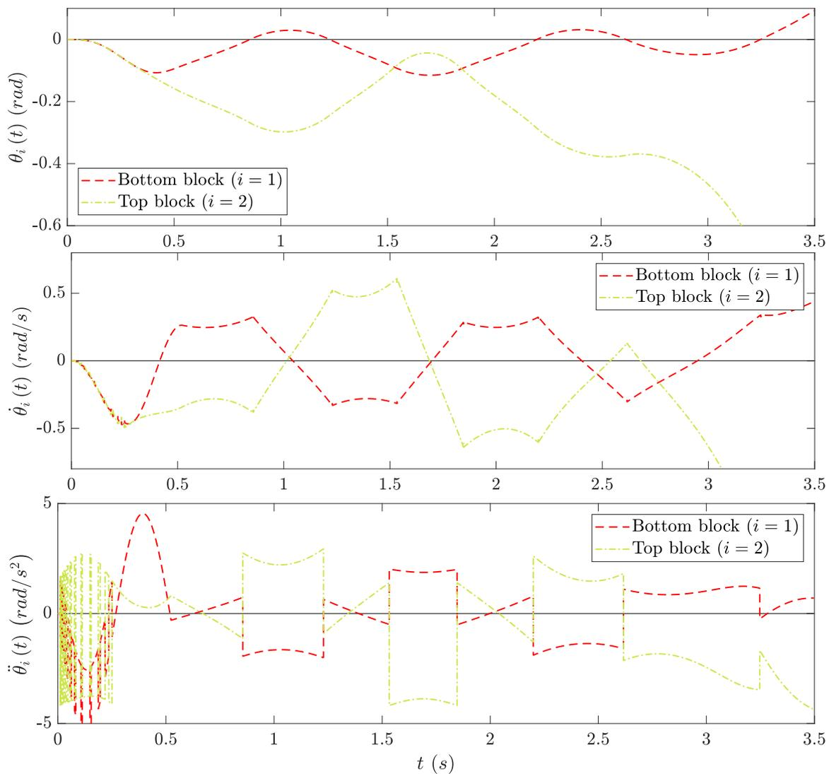
Figure 6.21: Rotation, angular velocity, and angular acceleration time histories for the dual-block stack subject to a single sine-wave excitation with  $a_0 = 10.7808g\alpha^*$  and  $\omega = 12$  rad/s
