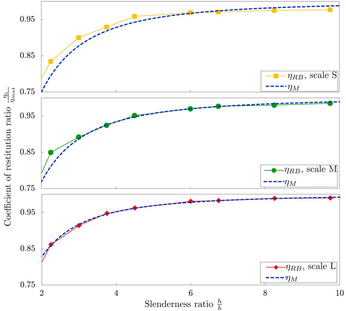
Figure 4.21: Coefficient of restitution  $\eta_{RB}$  and  $\eta_M$  [2, 3]
