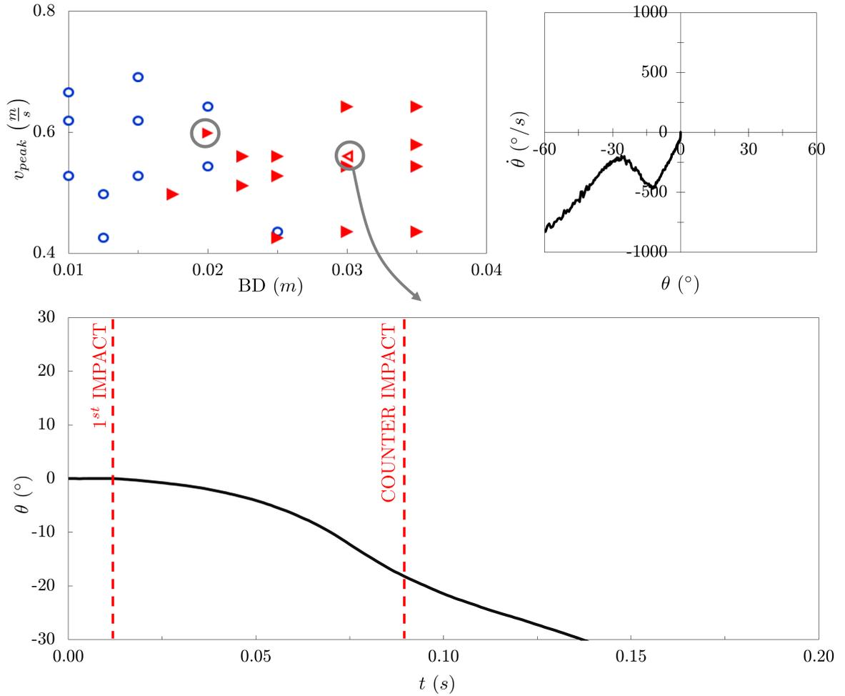
Figure 8.10: Phase plane view (above on the right) and rotation time history (below) of the experiment of a single block (Scale 1) motion with initial conditions  $v_{peak} = 0.56 \frac{m}{s}$ ,  $BD = 3.0 \text{ cm}$
