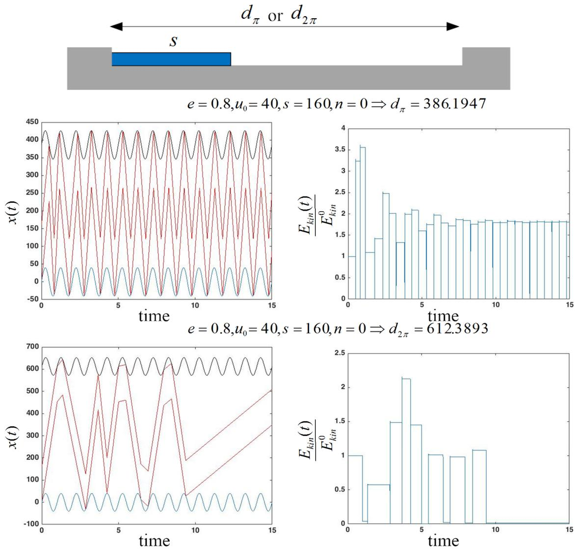
Figure 9.4: Trajectory and kinetic energy index time-histories for an intermediate restitution coefficient ( $1 > e > 0$ ) between the block and the moving boundary for the first collision at contact points  $(\pi, 2\pi)$
