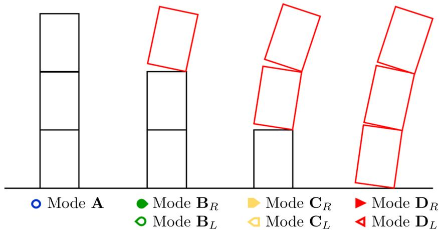
Figure 8.11: Modes of overturning of a three-block stack
