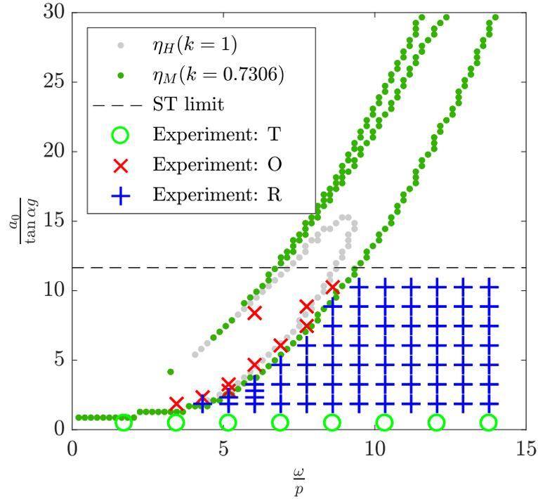
Figure 5.16: Stability graph due to a single sine wave for block B6L with  $h/b = 4.5$  (T - translation, O - overturning, R - rocking)
