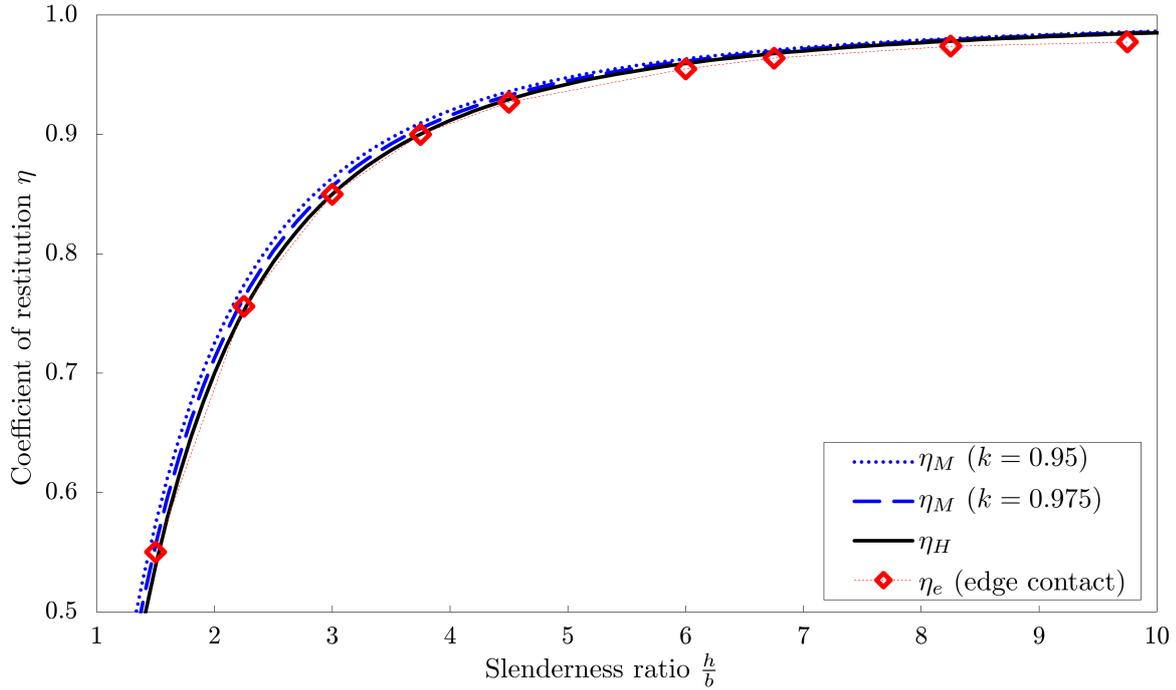
Figure 4.19: Coefficient of restitution obtained for blocks B1L - B10L (large scale,  $b = 6$  cm) with full- and edge-contact conditions
