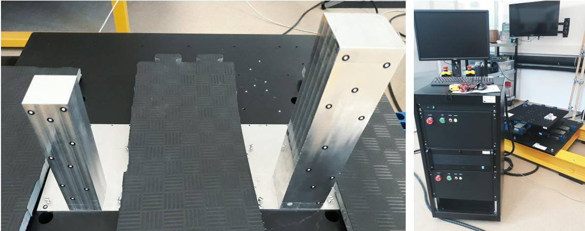
Figure 5.14: Two blocks of the same slenderness ratio but different size (left) on the shaking table system Quanser ST-III (right)
