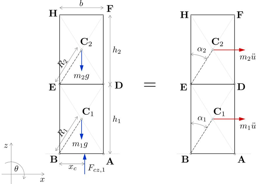
Figure 6.1: Free-body and mass-acceleration diagrams of a dual-block stack translating along with the base
