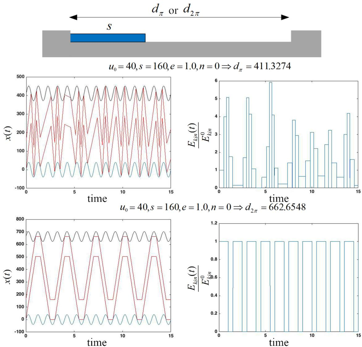
Figure 9.2: Trajectory and kinetic energy index time-histories for a fully elastic collision ( $e = 1$ ) between the block and the moving boundary for the first collision at contact points  $(\pi, 2\pi)$
