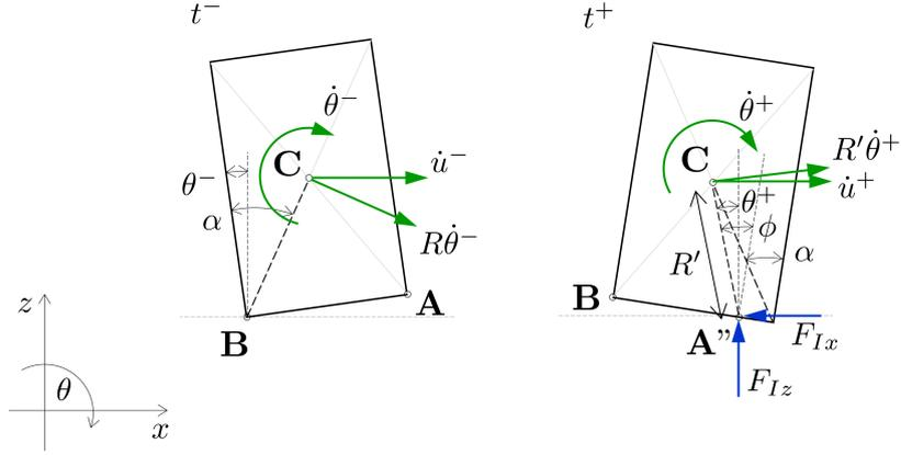
Figure 4.3: Pre-impact and post-impact velocity plans during transition from rocking around point B to rocking around an arbitrary point A”
