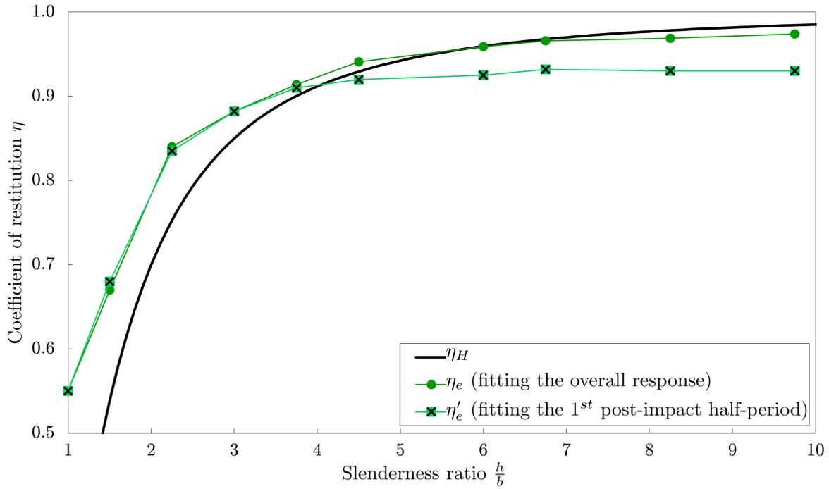
Figure 4.13: Coefficient of restitution from Housner's formula [1] and full-contact experiments for blocks B1M - B10M (medium scale) with different fitting
