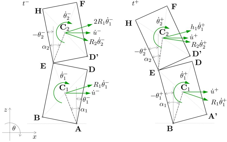
Figure 6.17: Velocity diagrams for configurations 2b and 1a
