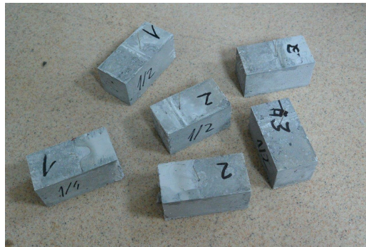
Figure 2.8: Six specimens containing a fiber: three with 1/4 embedded length, and three with 1/2 embedded length.
