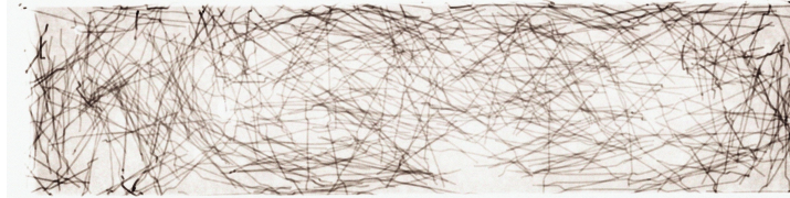
Figure 4.18: X-ray image of a fiber-reinforced concrete specimen [68].
