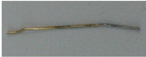
Figure 2.13: Fiber at the end of the analysis, where the straightening of the hook is visible on the pull-out side.
