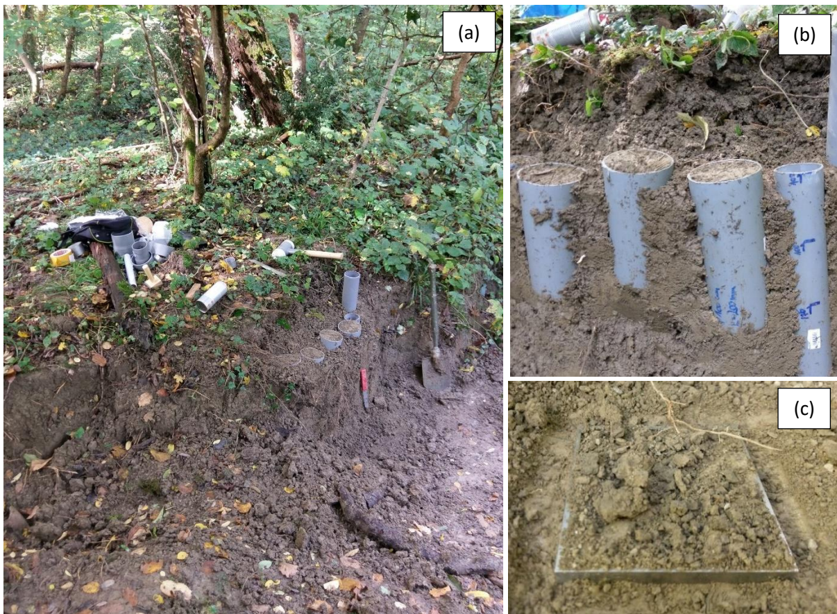
Figure 65: Some details on collection of undisturbed soil specimens from the a) sampling pit by insertion of b) hard plastic tubes or c) steel cutter for testing in direct shear apparatus.
