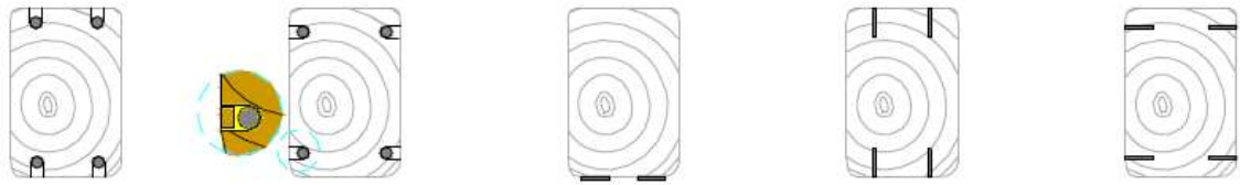
Figure 6.8 Strengthening measure with FRP strips [42]
