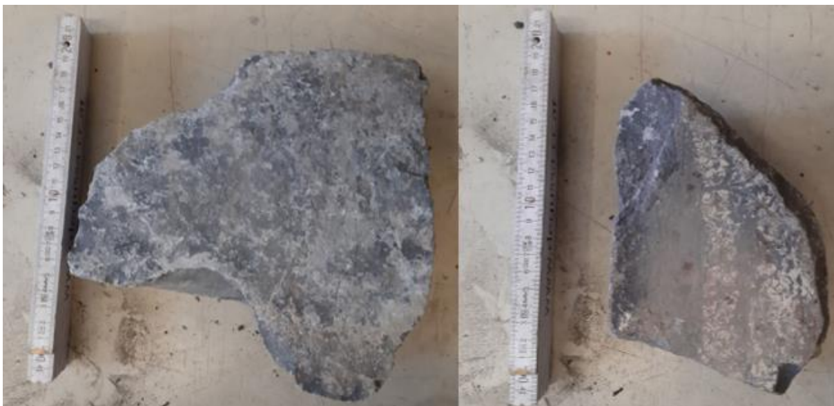
Figure 42 Basalt samples used for Schmidt hammer test
