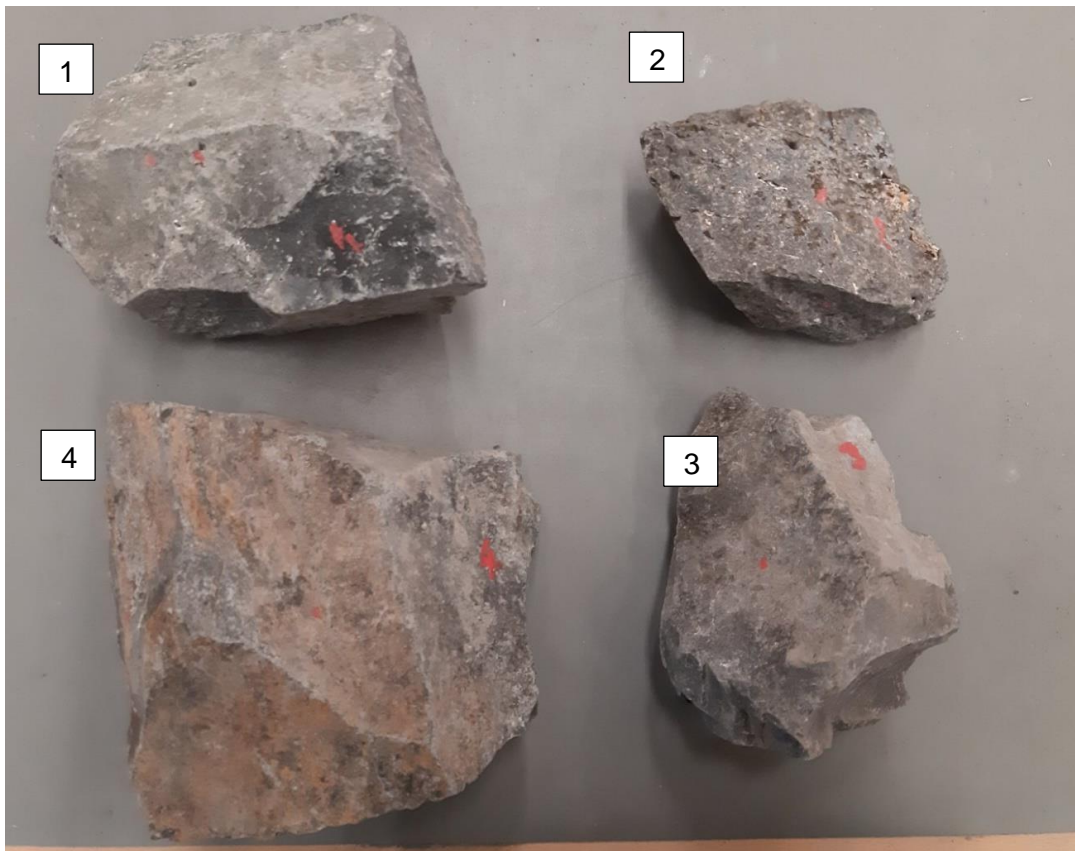
Figure 40 Basalt samples used for P-Wave velocity test.
