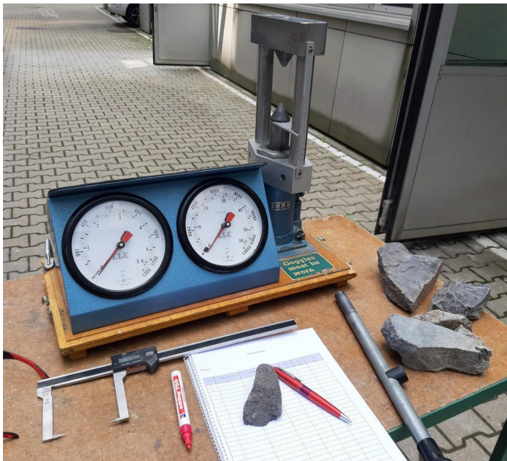
Figure 35 Point Load Test, device.
