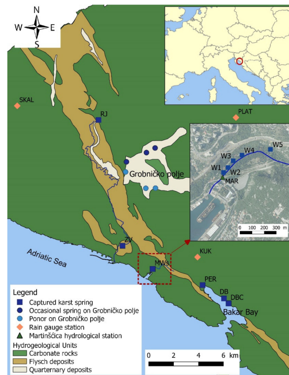
Figure 1. Upper right corner: position of the study area. The main map: hydrogeological map of the analyzed area showing the main karst springs (RJ)—Rječina Spring, ZV—Zvir, MWs—Martišćica wells,
