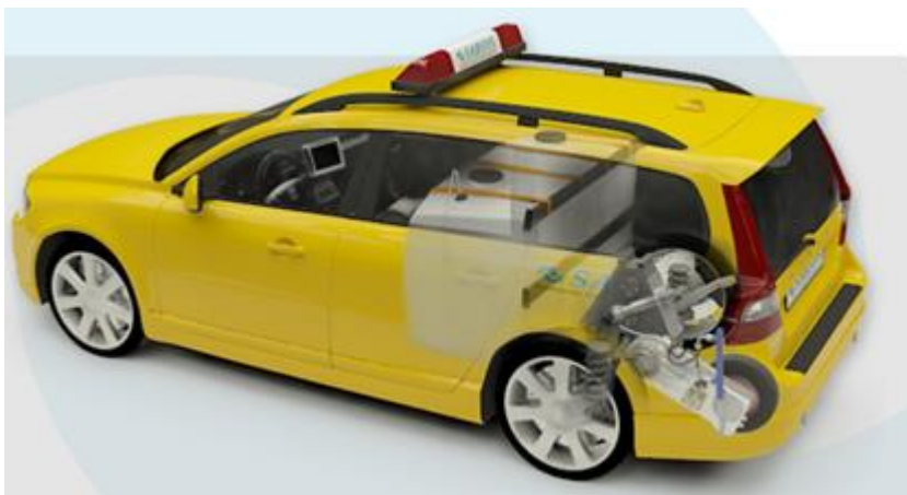
Slika 34. SARSYS Volvo friction tester (SVFT) [24]
