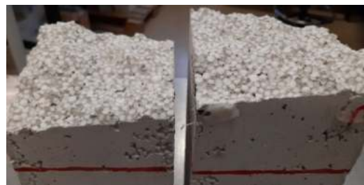
b) Failure surface
