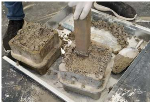
Figure 3. Casting of fresh concrete
