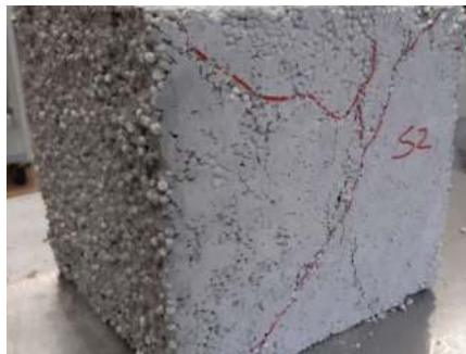
Figure 8. Compression test - failure patterns
