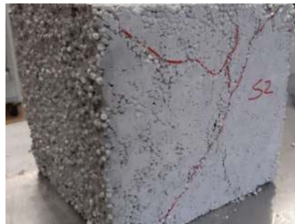
Figure 8. Compression test - failure patterns
