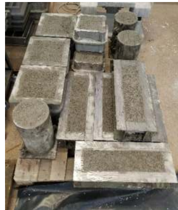
Figure 4. EPS3 concrete specimens
