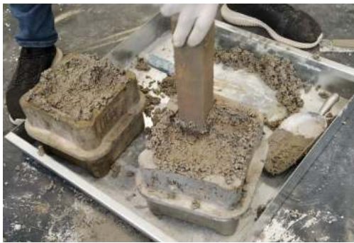
Figure 3. Casting of fresh concrete
