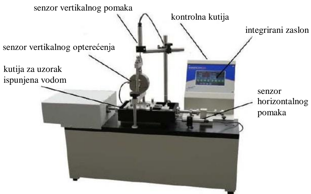
Slika 8: Uređaj za izravno smicanje (modificirano prema https://www.vjtech.co.uk/blog/an-introduction-to-direct-shear-testing )
