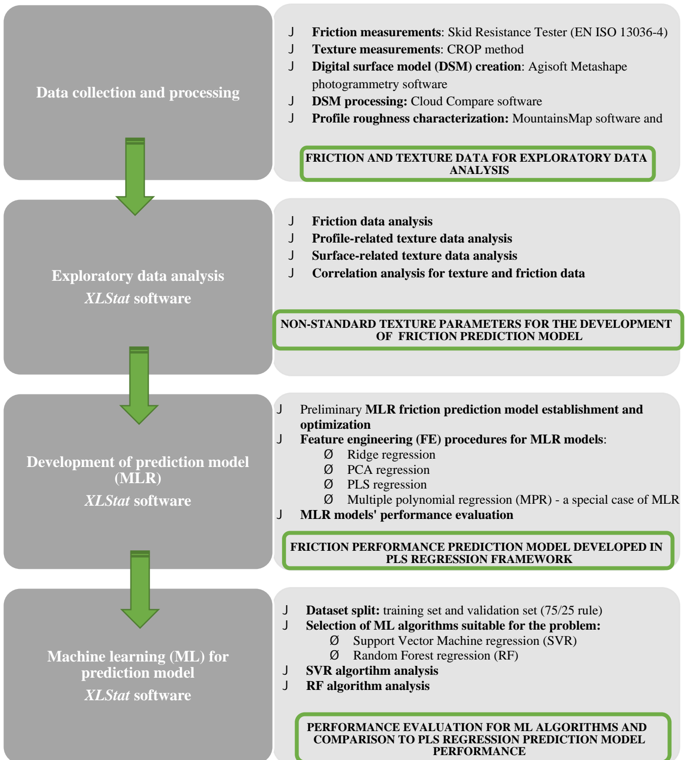
Figure 6.1 A schematic overview of performed procedures and used tools in the friction prediction model establishment
