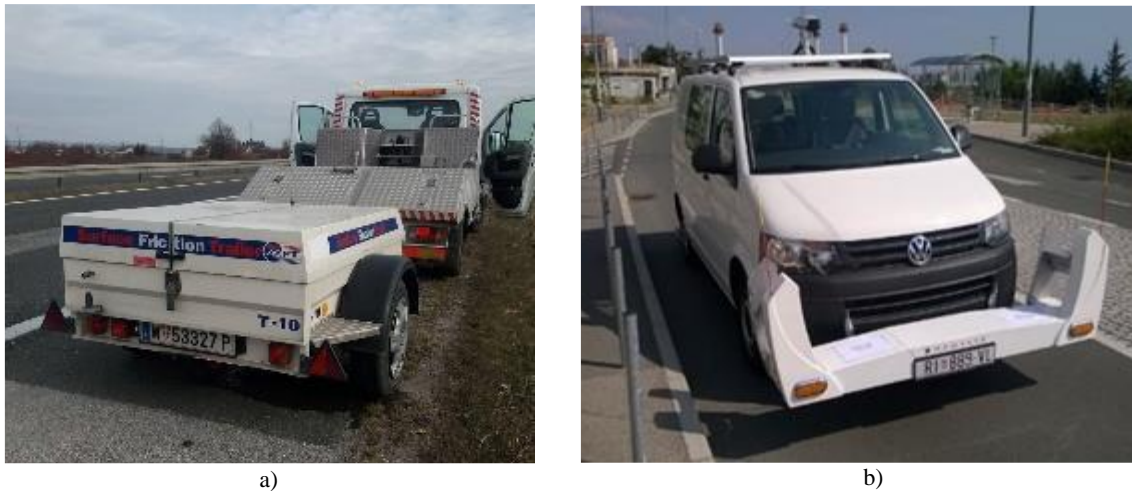
Figure 4.2. Data collection devices: friction measurement device (a) and texture measurement device (b)
