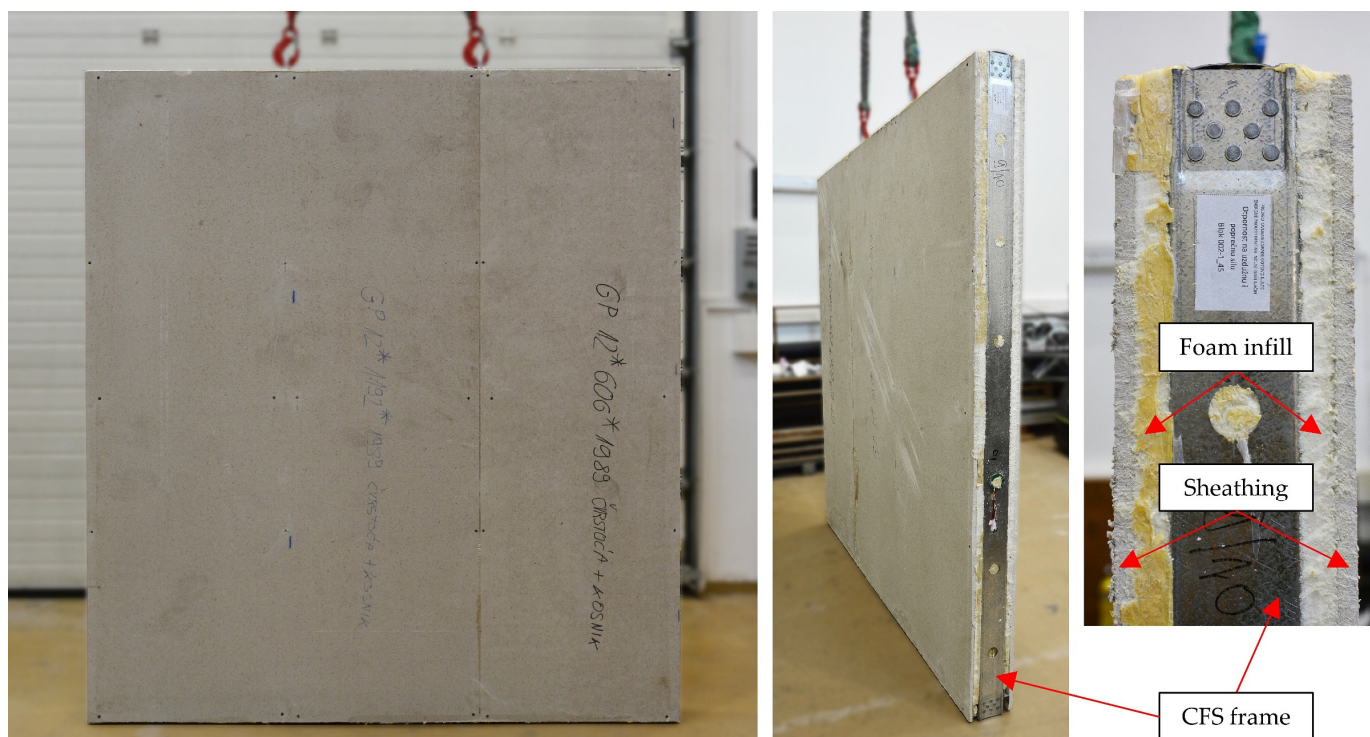
Figure 4. CFS-PU composite wall panel specimen with sheathings and PU foam filling.
