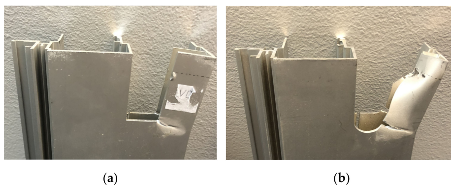
Figure 10. Fracture in monotonic tests: (a) Sharp notch specimen M_N1_1; (b) Semi-circular specimen M_N3.
