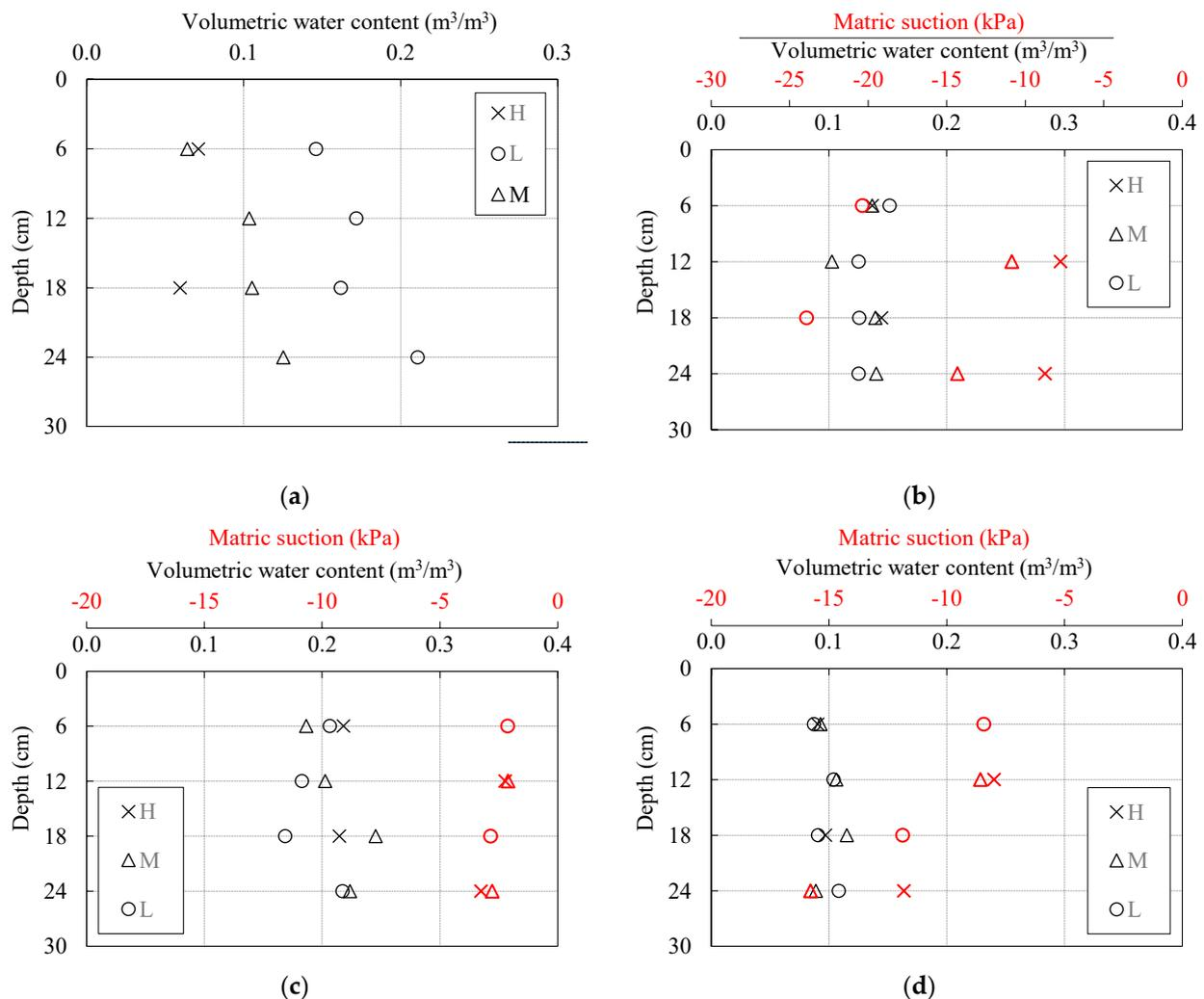
**Figure 14.** Initial volumetric water content and matric suction distributions along the upper (H), middle (M) and lower (L) measurement profiles for tests on 35-degree inclined slope models built in: (a) clean sand; (b) SK15; and SK10 with higher (c) and lower initial soil moisture contents (d).
