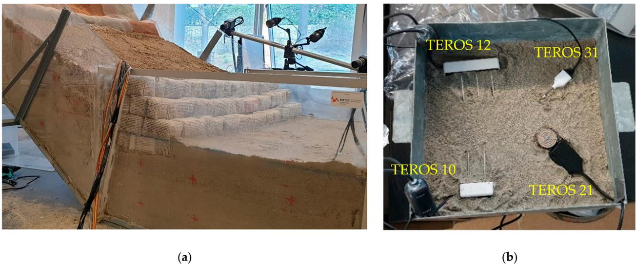
**Figure 5.** Details on (a) model setup with installation of sensors and cameras and (b) TEROS 12, 10, 31 and 21 sensors (top and bottom left and right, respectively) for hydraulic monitoring of slope models during the calibration procedure.
