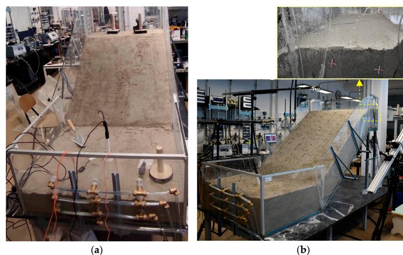
**Figure 1.** Some details of the model build-up: (a) compaction of the soil material with simultaneous installation of the measuring sensors; (b) scaled slope model with installed measuring equipment before the start of the test.
