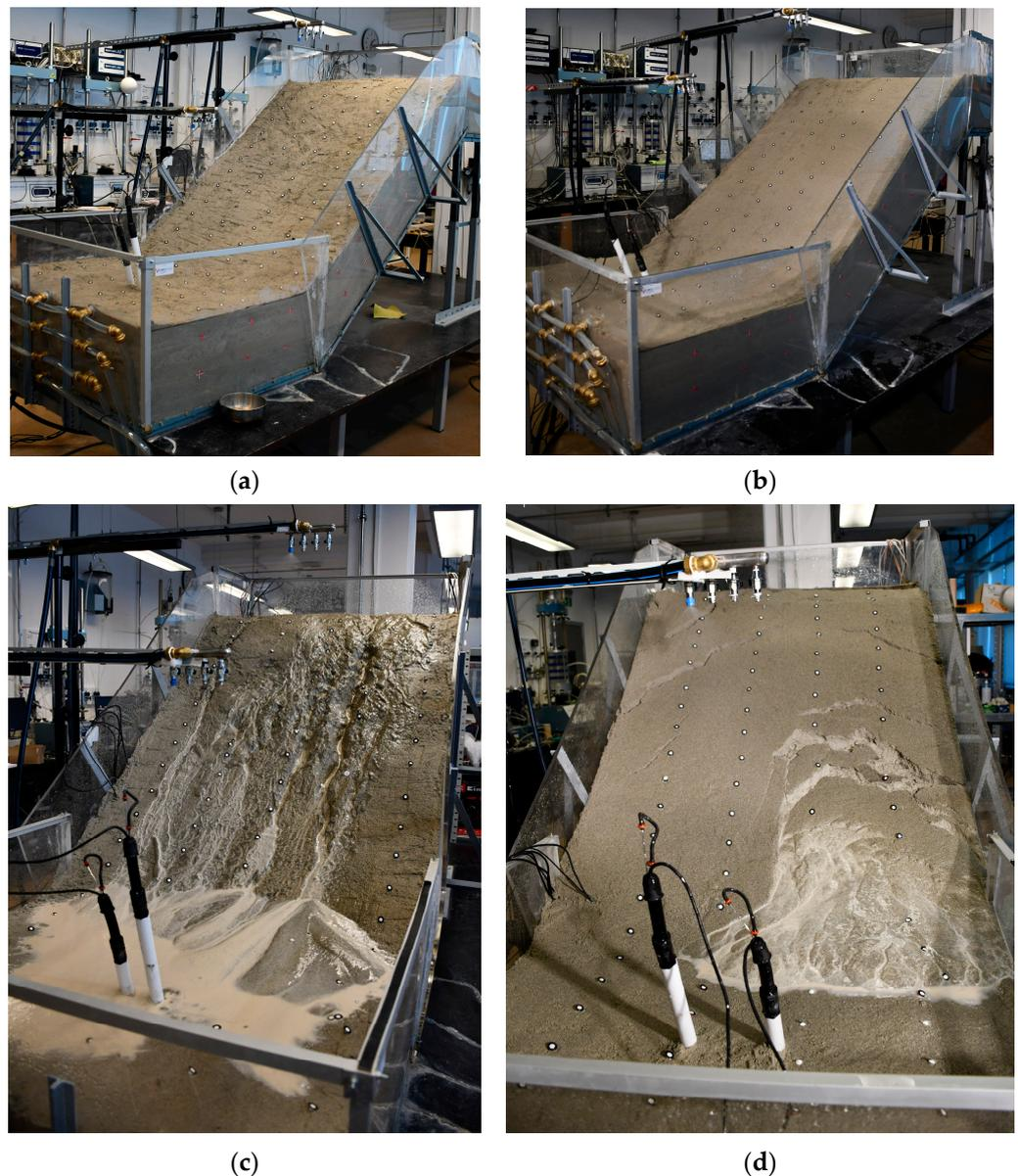
**Figure 15.** Two different types of instability depending on initial moisture in slope models: The slope model with higher initial moisture (a) leads to surface erosion (c), while the slope model with lower initial moisture (b) leads to the formation of cracks and landslides (d).
