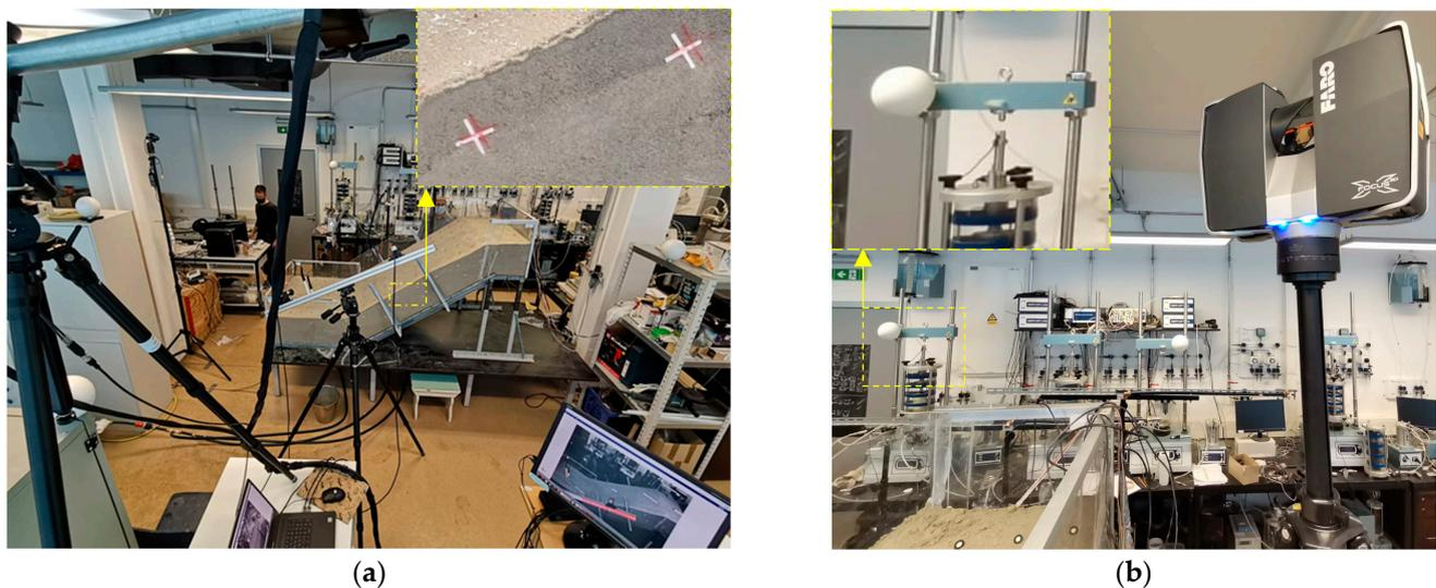
**Figure 3.** Geodetic monitoring equipment: (a) A view of the model from the ARAMIS measuring system (GOM mbH, Braunschweig, Germany) and a detail from the (front) 12-megapixel camera monitoring displacements through the plexiglass wall; (b) The FARO Focus 3D X 130 (FARO Technologies Inc, Lake Mary, USA) terrestrial laser scanner and a detail of the reference sphere location.
