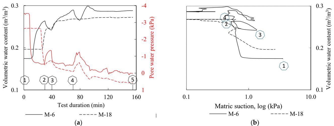
**Figure 12.** Hydraulic monitoring data from the test considered in Example 2 for points at 6 (M-6, continuous lines) and 18 cm depth (M-18, dashed lines) on the M measurement profile: (a) VWC and pore water pressure changes during the test; and (b) data in the logarithmic ( $u_a - u_w$ ) vs. VWC plane.
