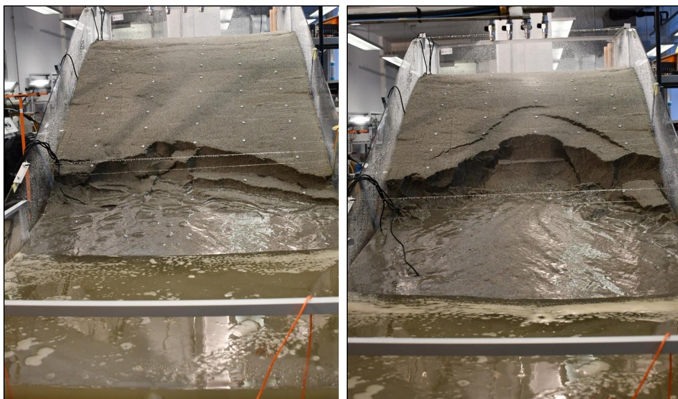
Figure 4. A photo of the Sand experiment around 90 min after the start of the rainfall simulation (left), showing the evolution of the retrogressive sliding following the formation of the rotational slide in the slope's toe, and a photo taken at the start of the surface runoff formation in the upper part of the model at around 125 min after the beginning of the Sand experiment (right).
