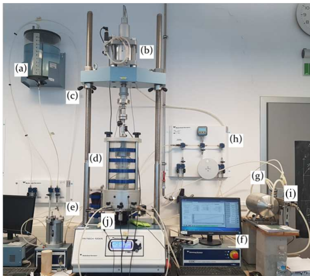
Figure 4. Cyclic triaxial system: (a) water tank, (b) pneumatic actuator, (c) triaxial loading frame, (d) triaxial cell, (e) volume controller, (f) PC with data acquisition system, (g) pneumatic control system for pressures and actuator, and (h) water distribution panel, according to [24].
