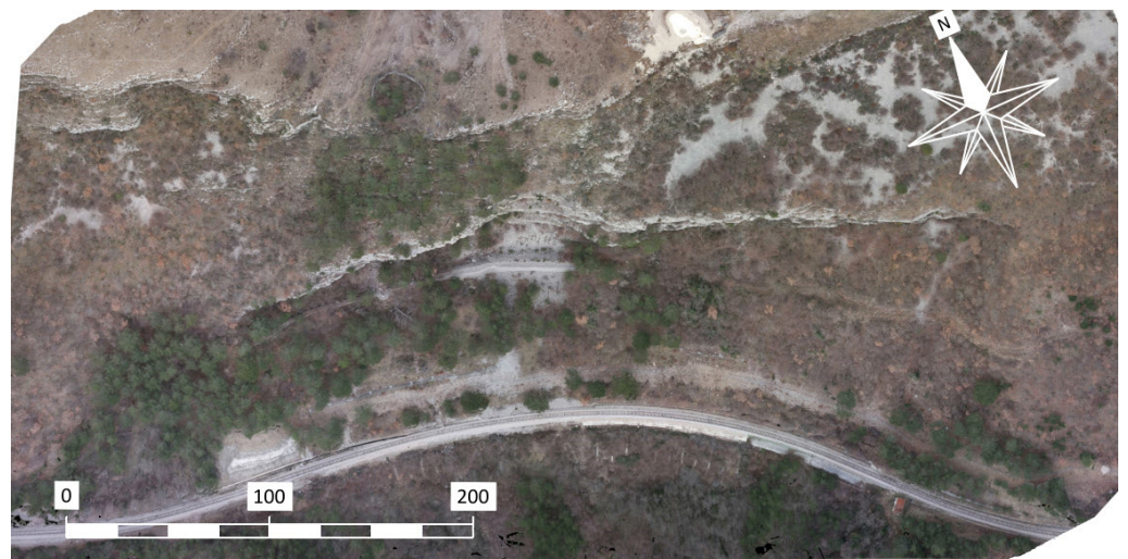
Figure 6. Orthophoto of Raspadalica Cliff derived from the SfM photogrammetry.
