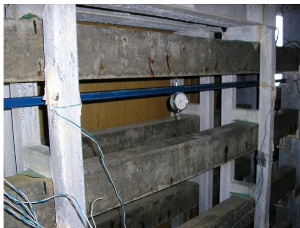
Figure 5. Beam specimens in the loading frame
