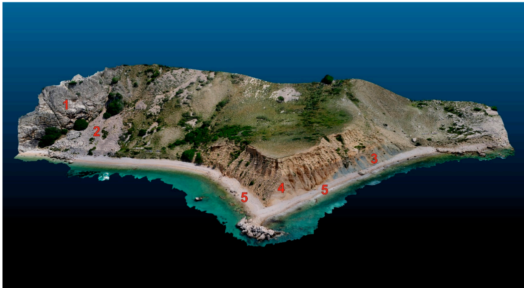
Figure 4. The wider area of Cape Pipa (photo: D. Kalajžić): 1—limestone rock, 2—active talus, 3—flysch (marls), 4—talus breccia; 5—beach body.
