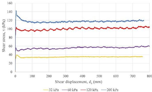
Figure 3. Shear stress-shear displacement of the RS tests.
