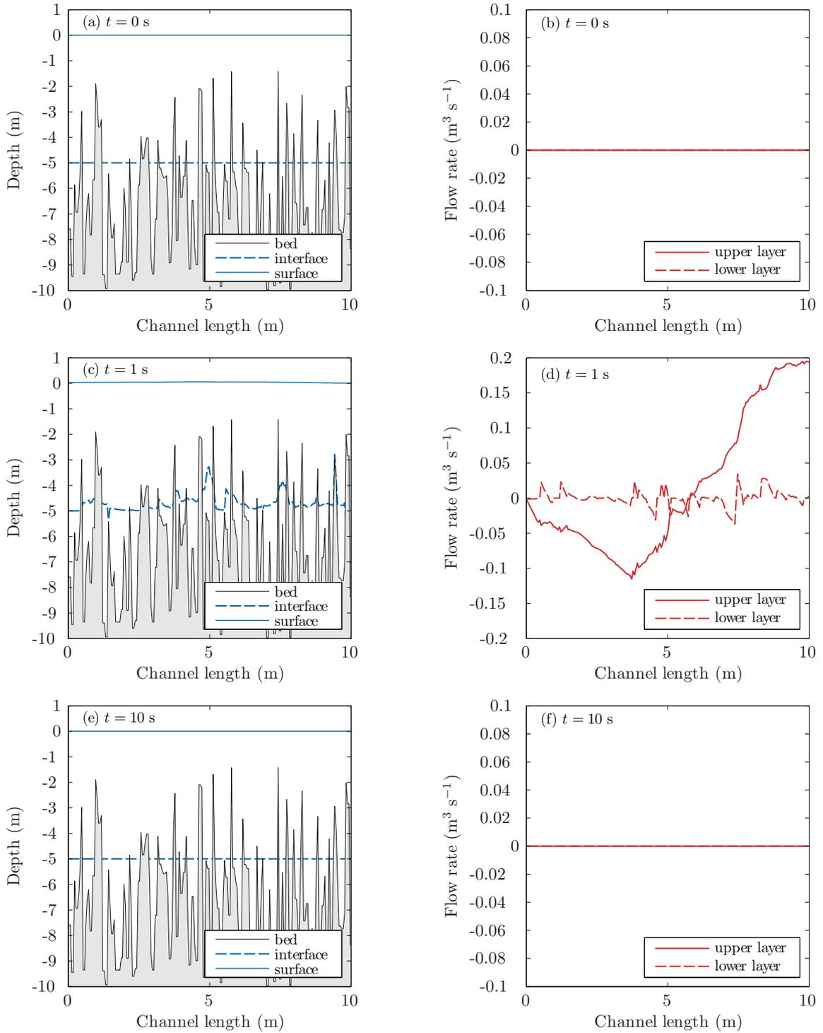
**Figure 5.6:** Extended C-property verification test for water at rest in an irregular channel with lower layer wet-dry transitions: (a) and (b) initial conditions (water depths and flow rates), (c) and (d) results at  $t = 1$  s when the original source terms are considered and spurious oscillations appear, and (e) and (f) results at  $t = 10$  s when the source term approximation is applied.
