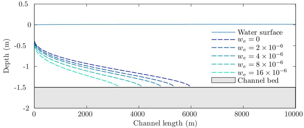
**Figure 5.9:** Sensitivity of the numerical model on the entrainment velocity  $w_e$  ( $\text{m s}^{-1}$ ), for  $Q = 2.0 \text{ m}^3 \text{ s}^{-1}$ ,  $\lambda_i = 10^{-3}$  and  $r = 0.975$ , without bed friction.
