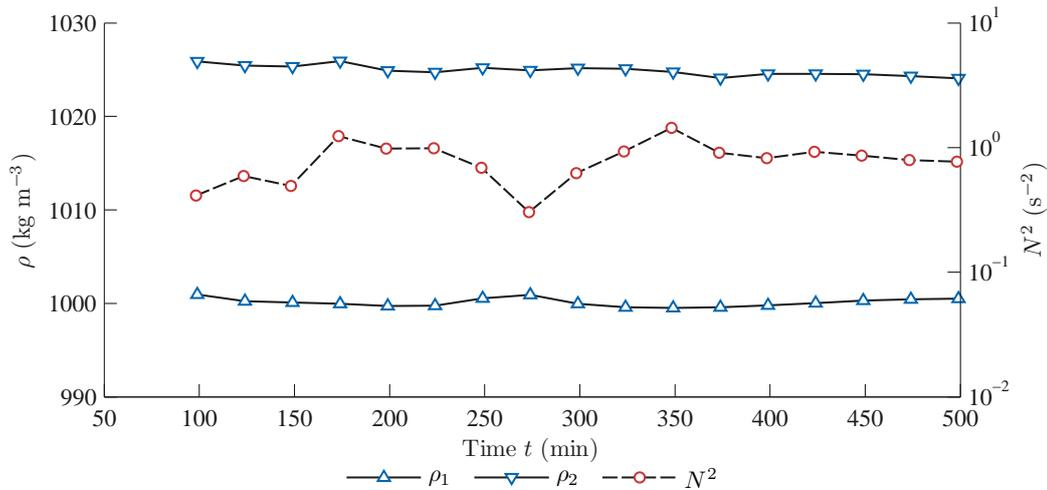
**Figure 8.6:** Observed density in the upper  $\rho_1$  and lower  $\rho_2$  layer and maximum squared buoyancy frequency  $N^2$ , averaged along the salt-wedge, during a simulation of a time-dependant flow observed on 1 July 2015.
