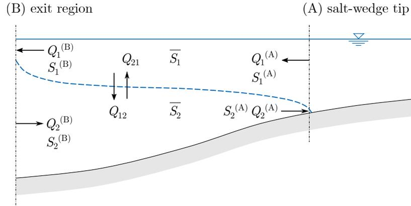
**Figure 6.10:** Scheme of a two-layer box model for estimating the vertical mixing in salt-wedge estuaries.
