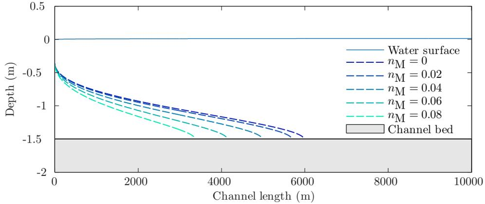
**Figure 5.8:** Sensitivity of the numerical model on the Manning's roughness coefficient  $n_M$ , for  $Q = 2.0 \text{ m}^3 \text{ s}^{-1}$ ,  $\lambda_i = 10^{-3}$  and  $r = 0.975$ , without entrainment.
