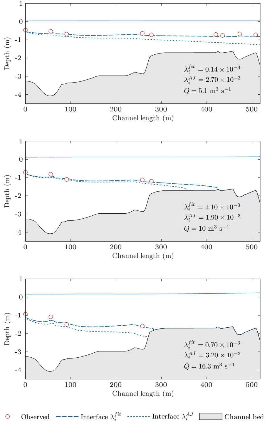
**Figure 7.2:** Numerical FDM solutions of the salt-wedge shape compared against field observations, for different river flow rates  $Q$ . Both  $\lambda_i^{fit}$  (fitted interfacial friction factor) and  $\lambda_i^{AJ}$  (computed from the Arita and Jirka model, Eq. (2.9)) were considered.
