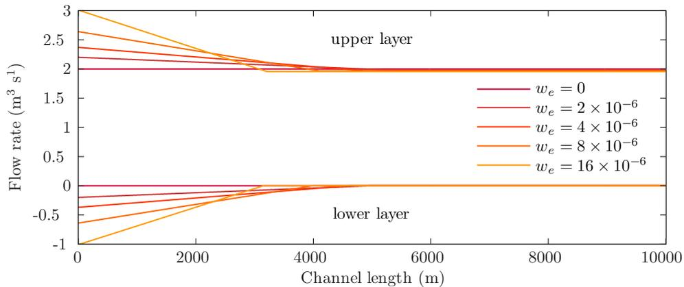
**Figure 5.10:** The resulting upper and lower layer flow rates for different entrainment velocities  $w_e$  ( $\text{m s}^{-1}$ ), for  $Q = 2.0 \text{ m}^3 \text{ s}^{-1}$ ,  $\lambda_i = 10^{-3}$  and  $r = 0.975$ , without bed friction.
