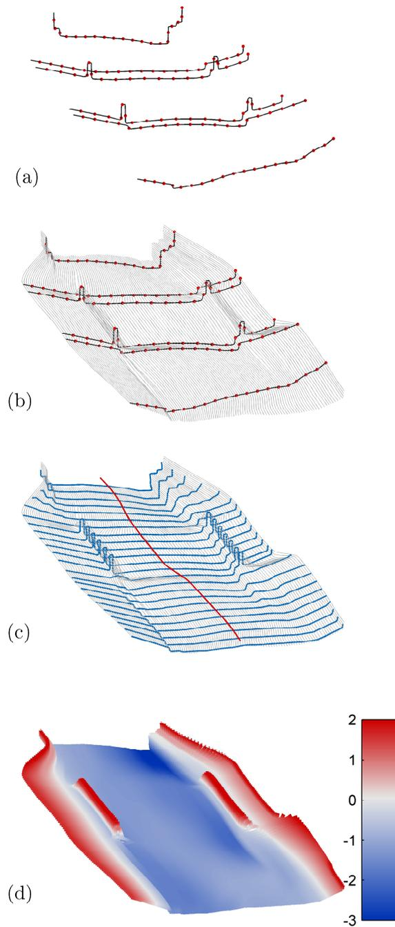
**Figure 6.14:** Step-by-step illustration of interpolation method for deriving DTM for a segment of the Rječina River estuary (from 0+440 m to 0+550 m): (a) measured cross sections, (b) interpolated profile lines, (c) interpolated cross sections along the centreline, and (d) digital terrain model.
