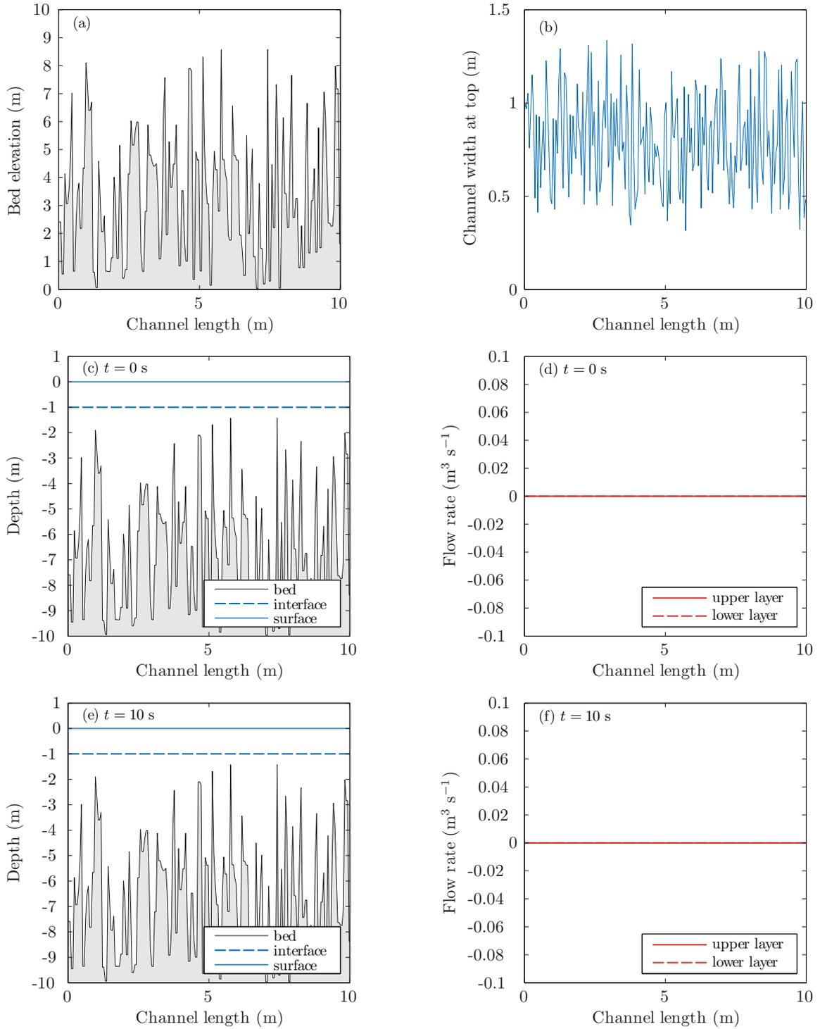
**Figure 5.5:** C-property verification test for water at rest in an irregular channel: (a) bed elevation, (b) channel width, (c) and (d) initial conditions (water depth and flow rate), and (e) and (f) results after  $t = 10$  s (water depths and flow rates).
