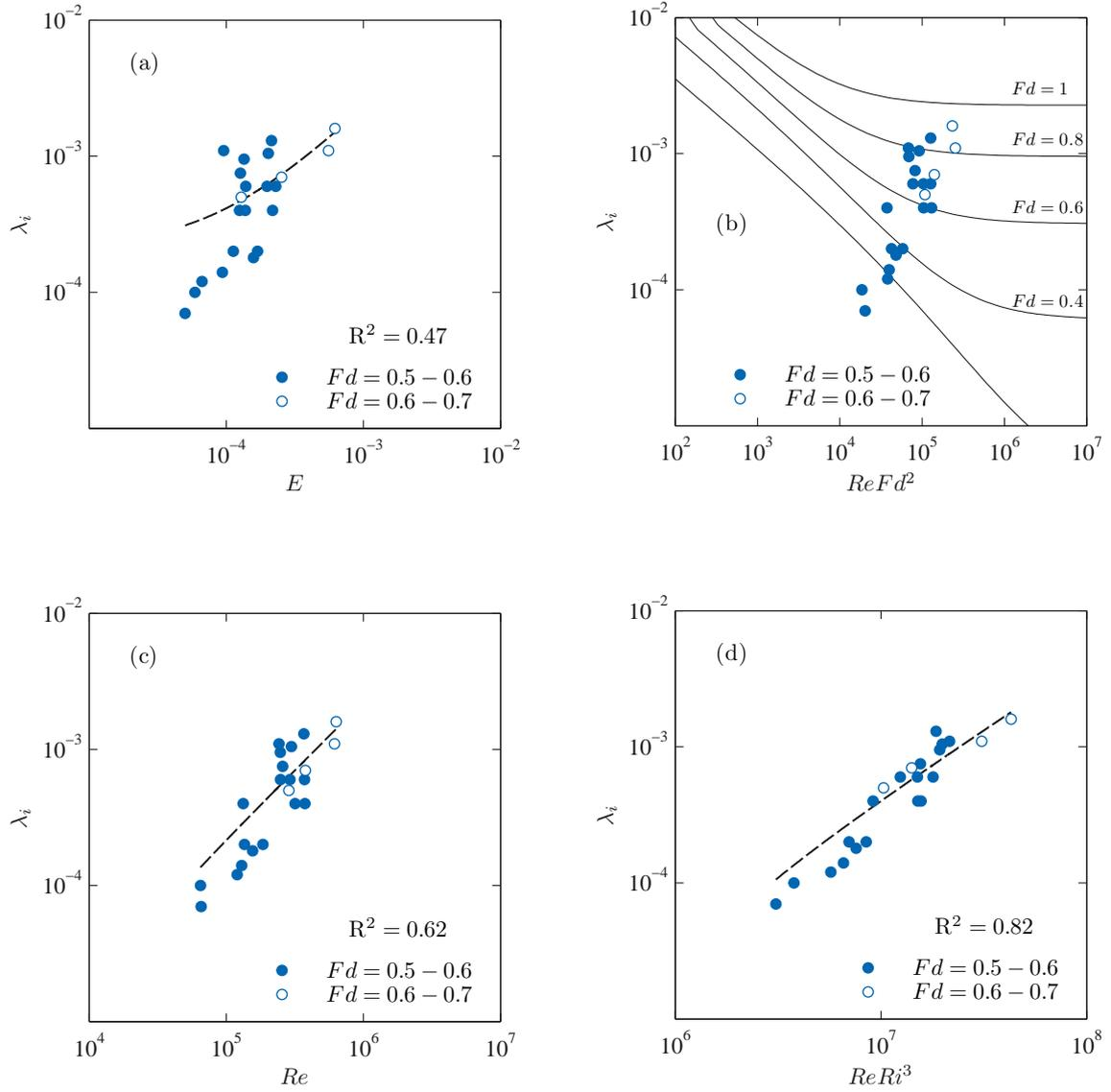
**Figure 8.4:** Dependence of the interfacial friction factor  $\lambda_i$  on: (a) entrainment rate  $E$ , Keulegan number  $ReFd^2$  with the Arita and Jirka model [2] (solid lines for different  $Fd$ ), (c) Reynolds number  $Re$  and (d) best fit combination of parameters  $ReRi^3$ .
