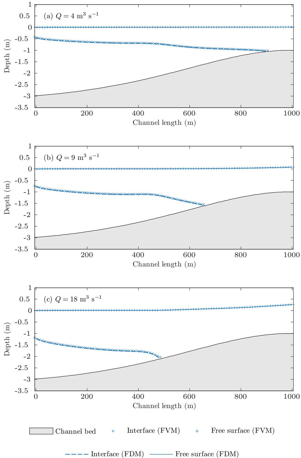
**Figure 5.4:** Numerical solutions for the arrested salt-wedge obtained by a steady FDM and a time-dependant FVM model, for (a)  $Q = 4 \text{ m}^3 \text{ s}^{-1}$ , (b)  $Q = 9 \text{ m}^3 \text{ s}^{-1}$  and (c)  $Q = 18 \text{ m}^3 \text{ s}^{-1}$ .
