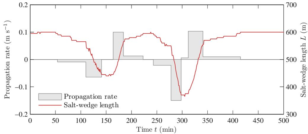
**Figure 8.7:** Computed movement of the salt-wedge front and corresponding propagation rates during the variable flow observed on 1 July 2015.
