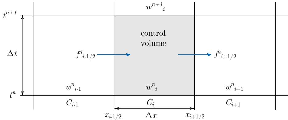
**Figure 4.3:** Graphical interpretation of a three-point explicit finite volume method.
