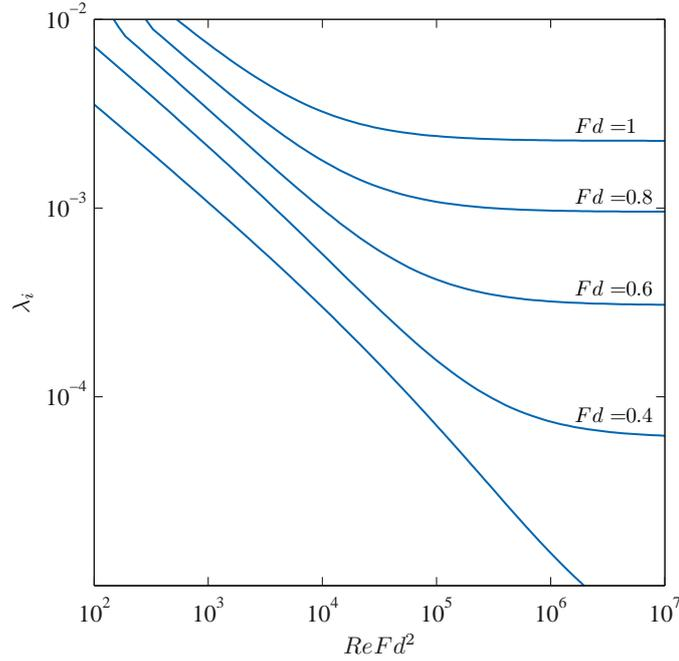
**Figure 2.2:** Arita and Jirka’s [2] friction law; interfacial friction factor  $\lambda_i$  dependence on  $ReFd^2$ .
