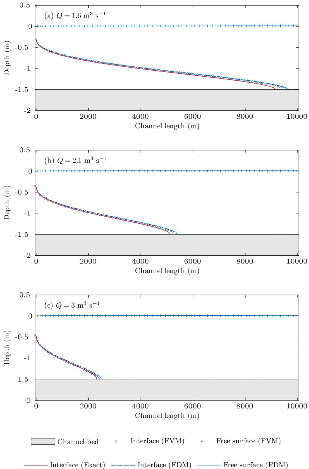
**Figure 5.2:** Numerical solutions for the arrested salt-wedge obtained by a steady FDM and a time-dependant FVM model, and their agreement with the exact solution for (a)  $Q = 1.6 \text{ m}^3 \text{ s}^{-1}$ , (b)  $Q = 2.1 \text{ m}^3 \text{ s}^{-1}$  and (c)  $Q = 3.0 \text{ m}^3 \text{ s}^{-1}$ .
