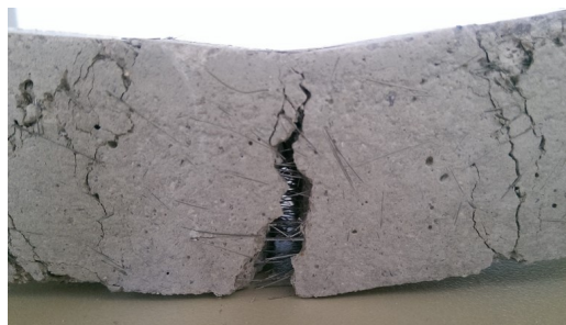
Figure 1.1: Crack in a fiber-reinforced concrete specimen at the end of a three-point bending test, with fibers bridging the notch.
