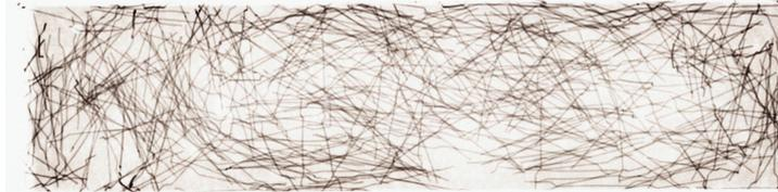
Figure 4.18: X-ray image of a fiber-reinforced concrete specimen [68].
