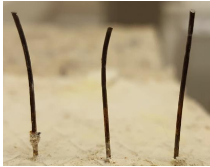
Figure 3.35: Steel fibers at the end of the test [41].
