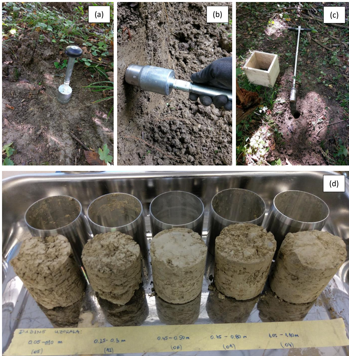
Figure 7: Collection of near-surface soil samples by using the equipment for undisturbed soil sampling (Eijkelkamp Soil&Water, Inc.) for determination of natural water content and basic physical properties. Sampling depths (0.05; 0.25; 0.45; 0.75; and 1.05 m) are indicated below samples in Figure 7 d).
