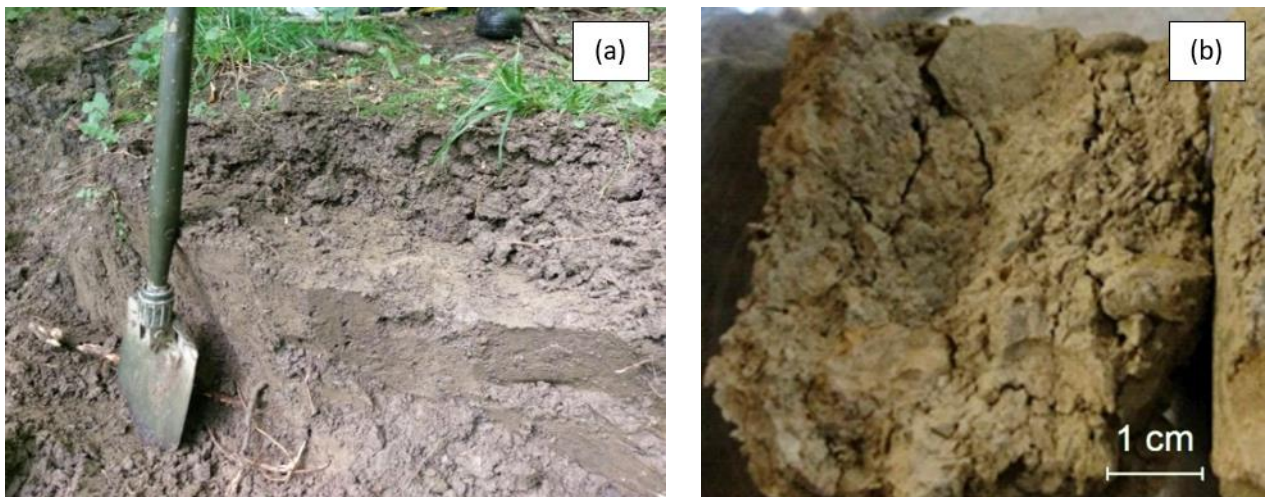
Figure 3: a) Sampling pit; b) half of the oven-dried specimen from a depth of 0.75 m.
