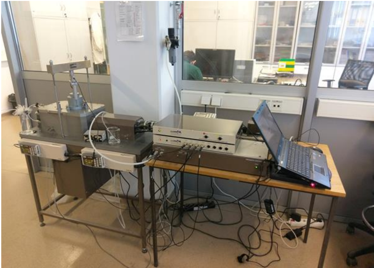
Figure 81: Back pressurized direct shear apparatus for soil testing in unsaturated conditions (GDS Instruments Ltd.) in Geotechnical laboratory of Faculty of Civil Engineering, UniRi.
